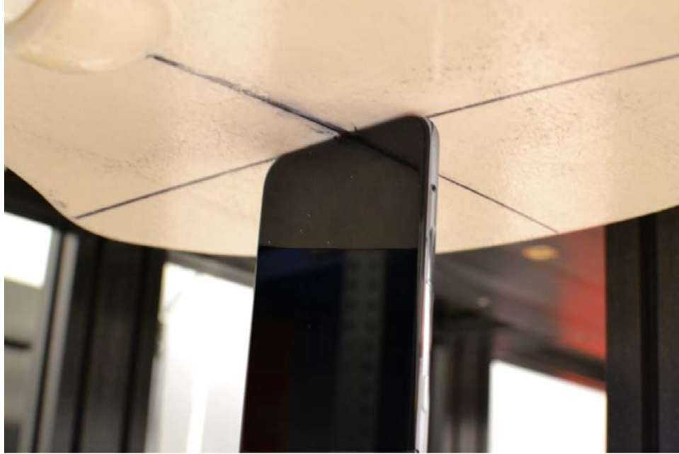
SAR Test Setup Photo 15- Bottom Edge at 0 mm
