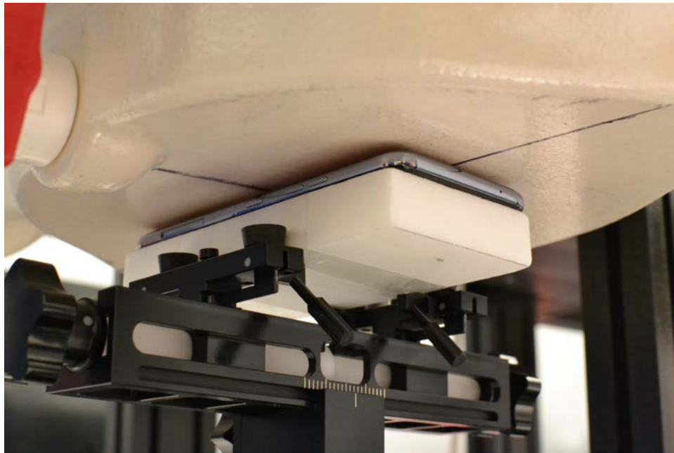
SAR Test Setup Photo 6- Back Side at 2 mm
