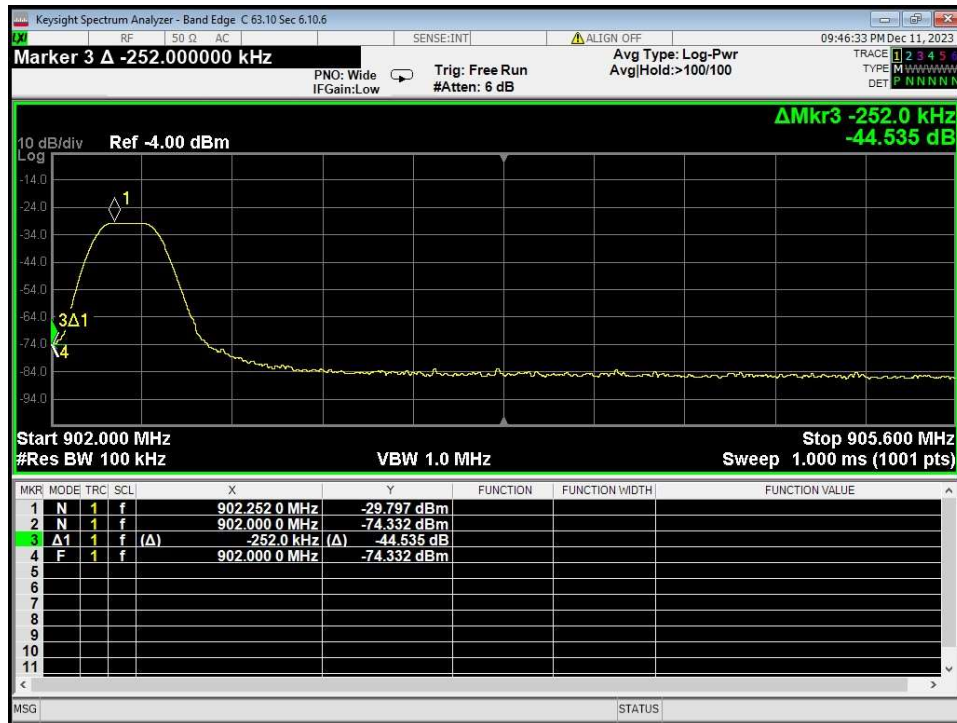
Figure 14 –Band-edge Measurement, Low Channel, Unrestricted Frequency
