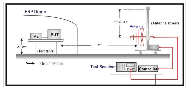
Above 1GHz Test Setup:
