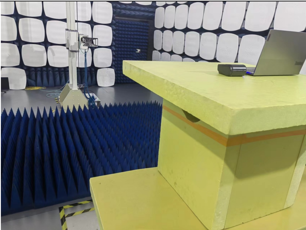
Radiated emission Test Setup (Above 1GHz)
