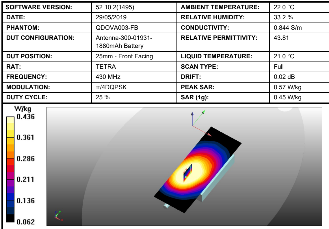
Figure 5: SAR Front Of Face Testing Results for the SC2124 at 430 MHz.
