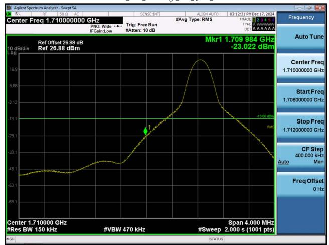
LTE B4\_15 M\_Band Edge\_Low\_QPSK\_1RB
