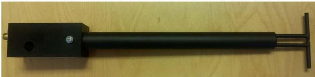
Figure 1 – MVG COMOSAR Validation Dipole
