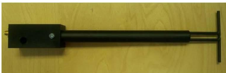
Figure 1 – MVG COMOSAR Validation Dipole
