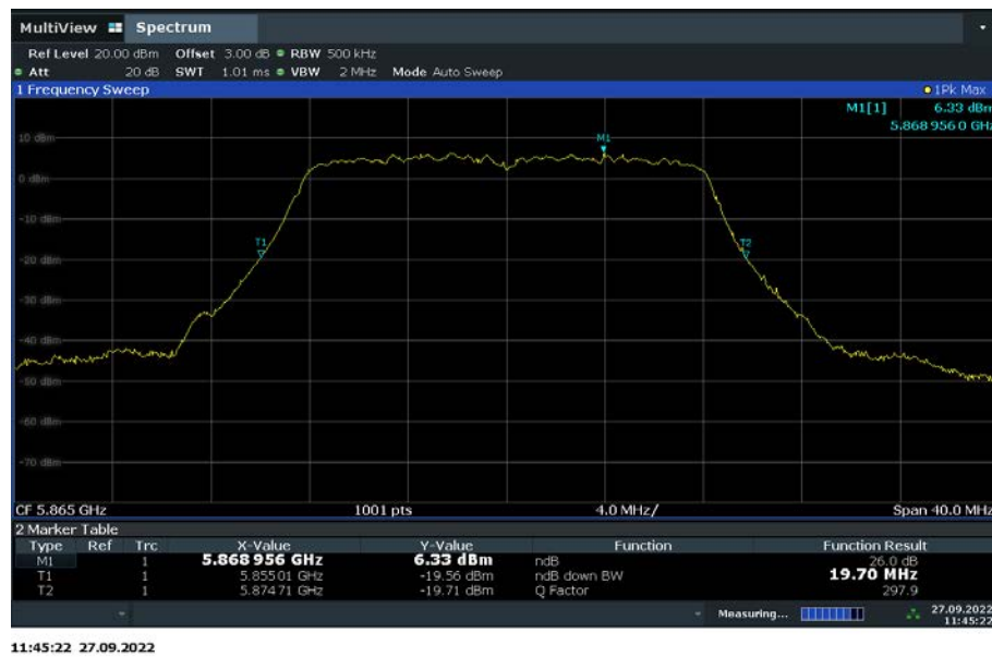
Fig. 78 Occupied 26dB Bandwidth (802.11a, channel 173)
