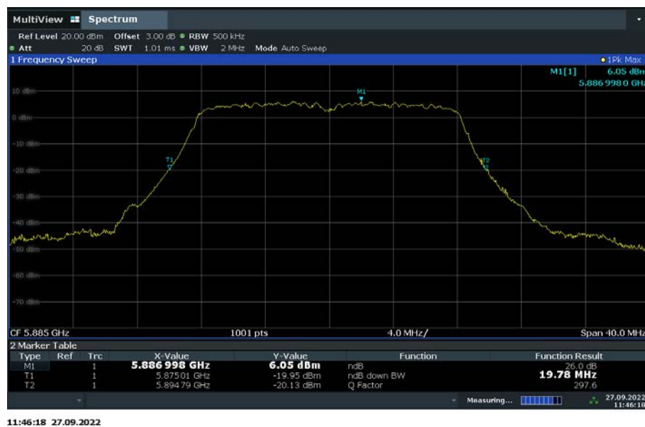
Fig. 79 Occupied 26dB Bandwidth (802.11a, channel 177)
