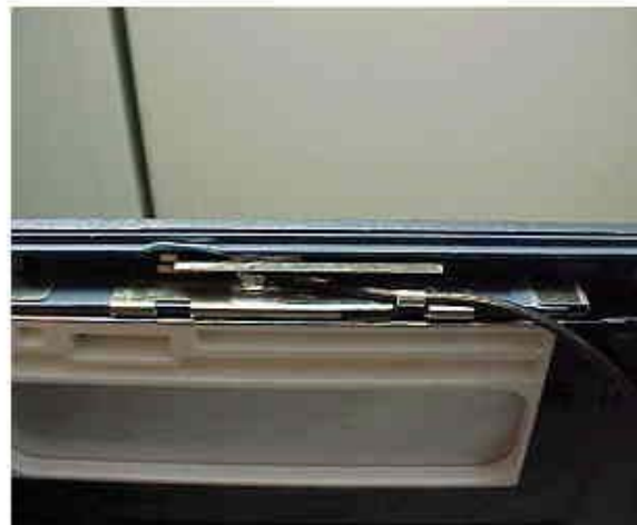
Fig-1 Left side antenna
