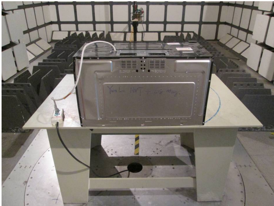
Radiated Emissions - Rear View (Above 1 GHz)
