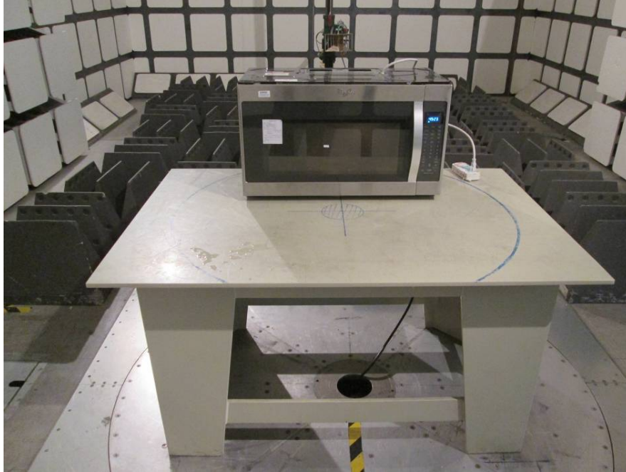
Radiated Emissions - Front View (Above 1 GHz)
