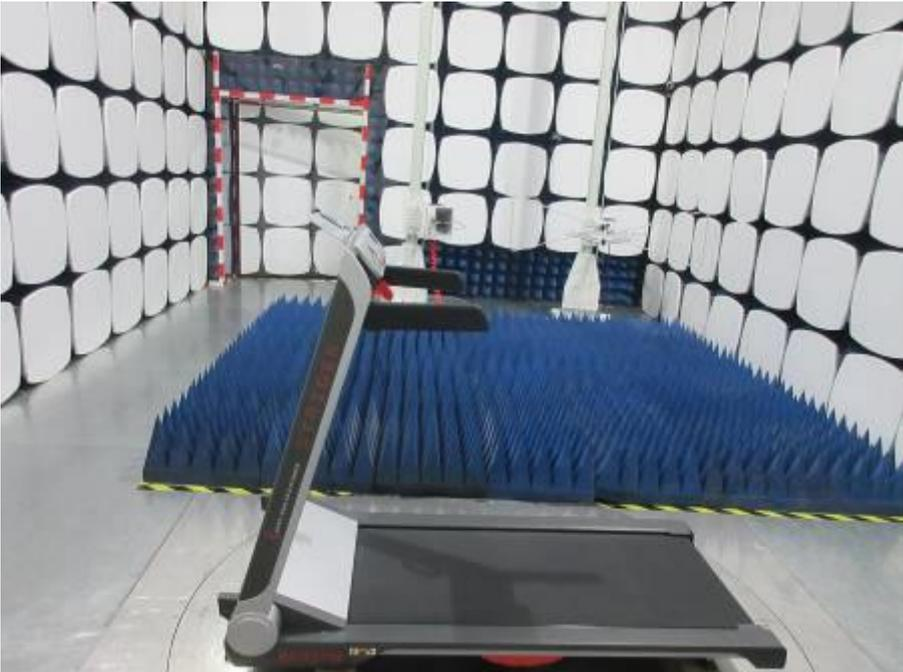
1.4 Radiated Spurious Emissions Test Setup
