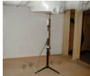
Figure 12.1 Dipole Validation Test Setup
