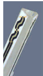
Figure 3.2 Probe Thick-Film Technique
