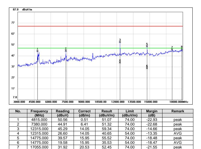
Note: 1. Reading +Correct (Amplifier Factor + Cable Loss + Antenna Factor + High Pass Filter Loss Factor)
