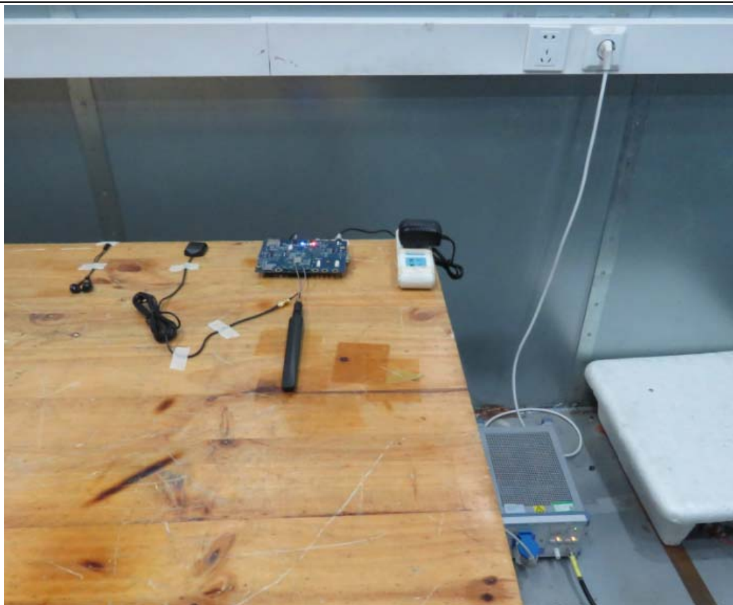
Picture 3: AC Power Line Conducted Emissions Test setup
