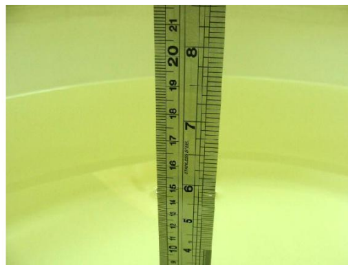
Fig 7.2 Photo of Liquid Height for Body SAR
