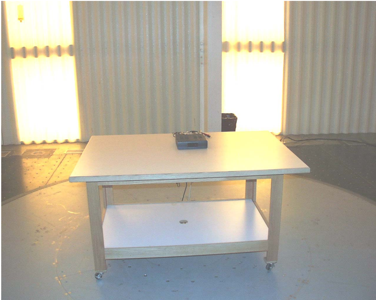
Photograph 1 - Front View Spurious Radiated Emission Worst Case Configuration
