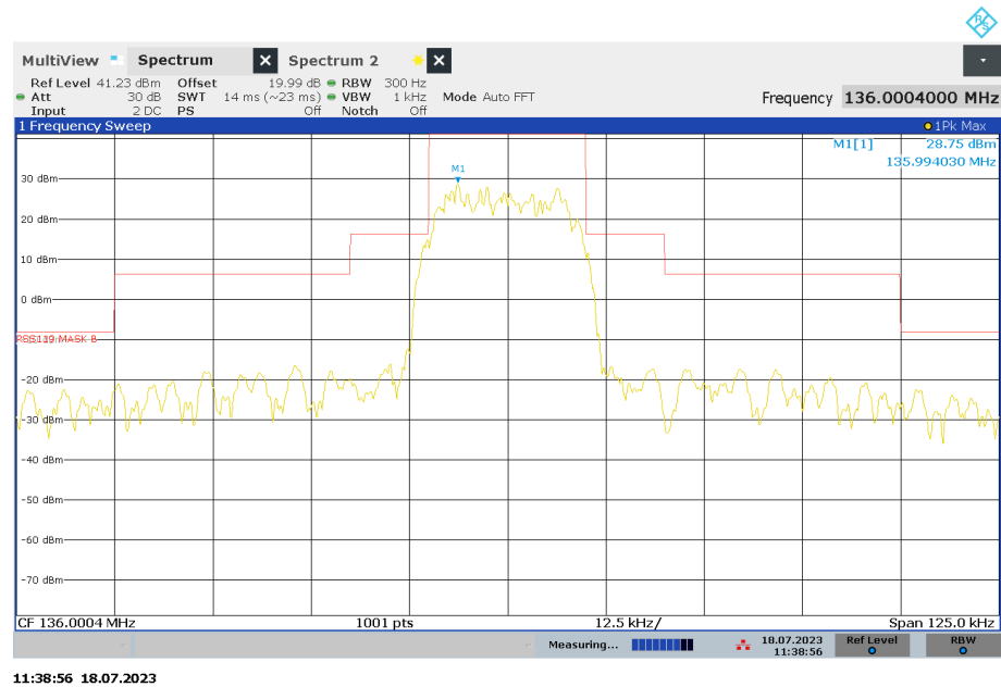
Figure 7 - 136 MHz, Transmitter Mask
