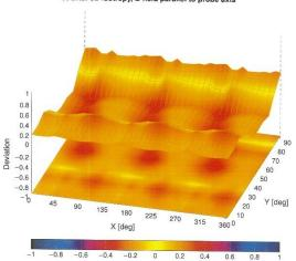
Probe isotropy for E<sub>tot</sub>: probe rotated  $\phi$  = 0° to 360°, tilted from field propagation direction  $\tilde{k}$  Parallel to the field propagation ( $\psi$  = 0° - 90°) at 30 GHz: deviation within  $\pm$ 0.43 dB Parallel to the field propagation ( $\psi$  = 0° - 90°) at 60 GHz: deviation within  $\pm$ 0.35 dB
