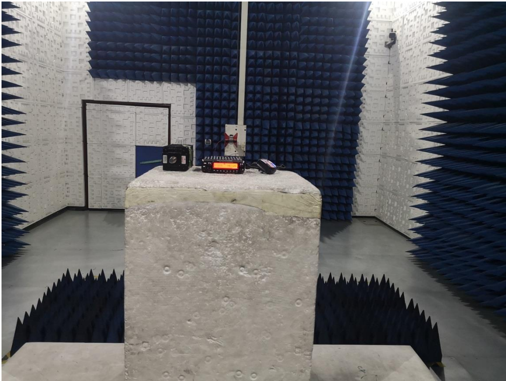
RADIATED EMISSION TEST SETUP ABOVE 1GHZ
