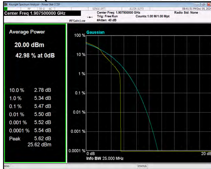
Band25 16QAM BW=15MHz Channel=26115 RB Size=1 Position=#0
