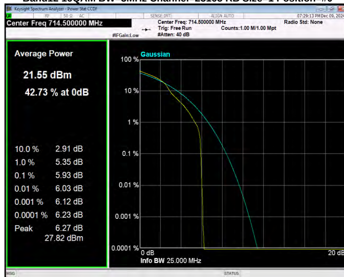
Band12 16QAM BW=3MHz Channel=23025 RB Size=1 Position=#0
