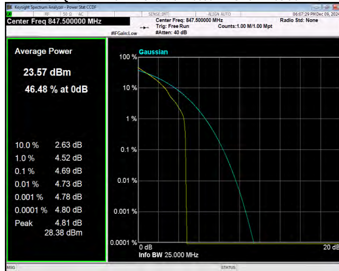
Band5 QPSK BW=5MHz Channel=20625 RB Size=1 Position=#0
