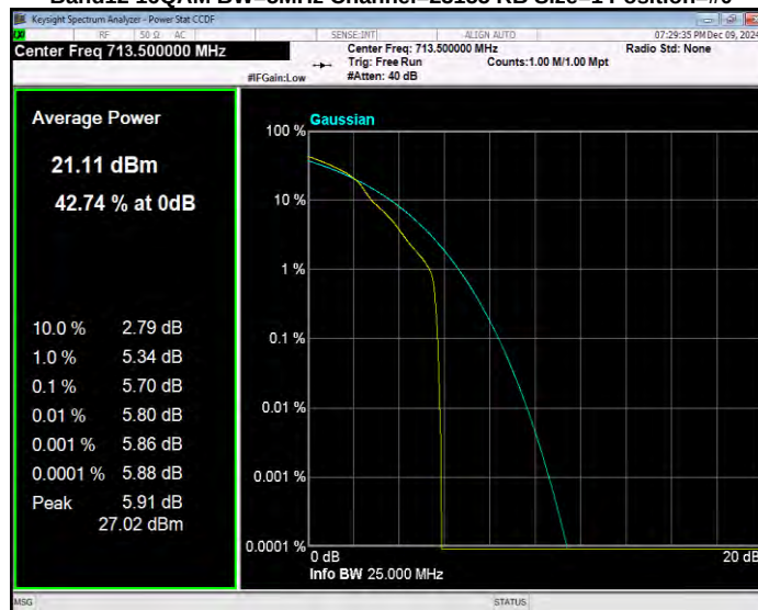
Band12 QPSK BW=3MHz Channel=23025 RB Size=1 Position=#0
