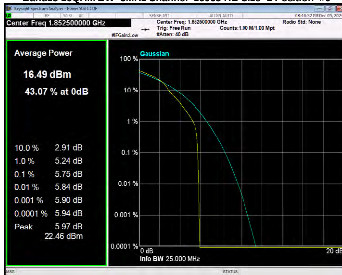
Band25 16QAM BW=5MHz Channel=26365 RB Size=1 Position=#0
