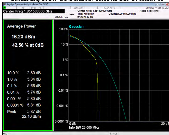
Band25 16QAM BW=3MHz Channel=26365 RB Size=1 Position=#0
