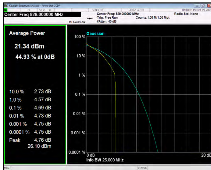
Band5 QPSK BW=1.4MHz Channel=20643 RB Size=1 Position=#0
