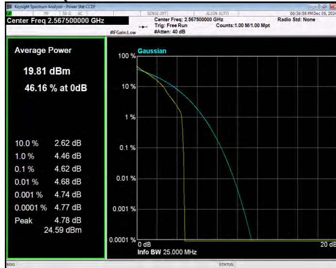
Band12 16QAM BW=1.4MHz Channel=23173 RB Size=1 Position=#0
