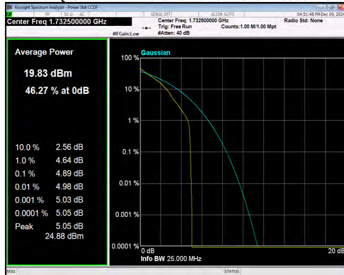
Band4 QPSK BW=15MHz Channel=20325 RB Size=1 Position=#0
