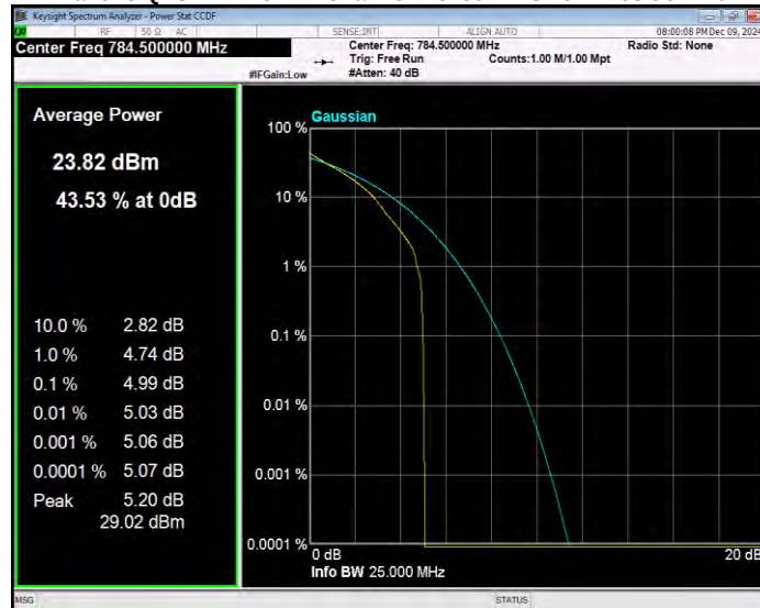
Band13 16QAM BW=5MHz Channel=23230 RB Size=1 Position=#0
