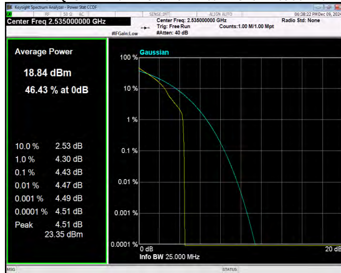
Band7 QPSK BW=20MHz Channel=21350 RB Size=1 Position=#0
