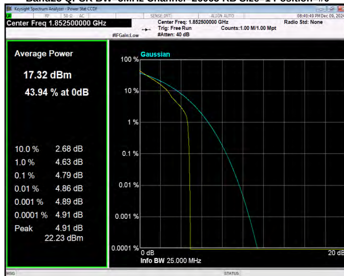
Band25 QPSK BW=5MHz Channel=26365 RB Size=1 Position=#0
