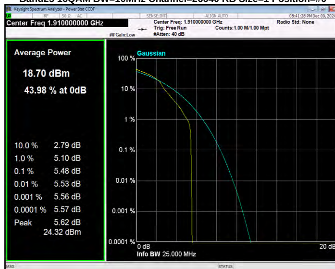
Band25 16QAM BW=3MHz Channel=26055 RB Size=1 Position=#0
