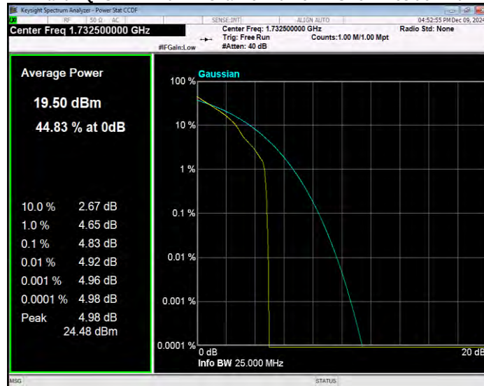
Band4 QPSK BW=1.4MHz Channel=20393 RB Size=1 Position=#0
