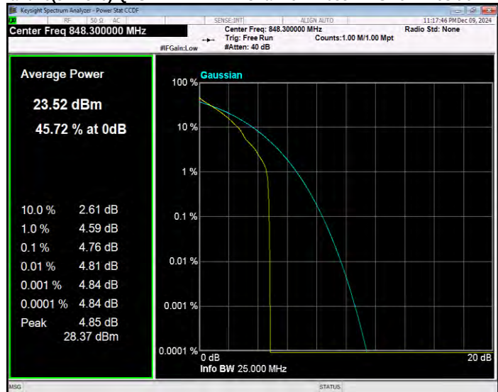
Band26(824-849) QPSK BW=10MHz Channel=26840 RB Size=1 Position=#0
