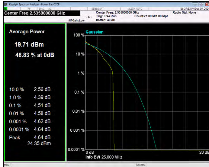
Band7 QPSK BW=15MHz Channel=21375 RB Size=1 Position=#0
