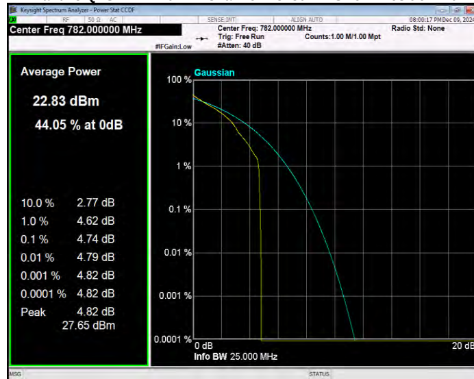
Band25 16QAM BW=1.4MHz Channel=26683 RB Size=1 Position=#0
