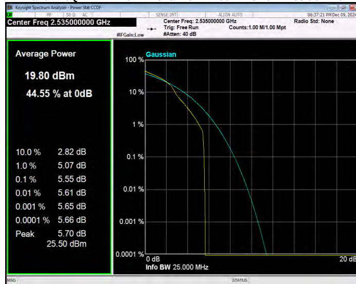
Band7 16QAM BW=15MHz Channel=20825 RB Size=1 Position=#0
