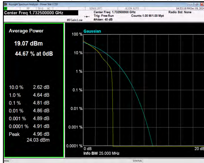
Band4 QPSK BW=10MHz Channel=20350 RB Size=1 Position=#0
