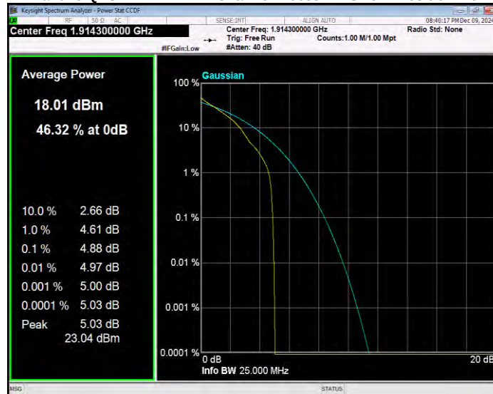
Band25 QPSK BW=10MHz Channel=26090 RB Size=1 Position=#0
