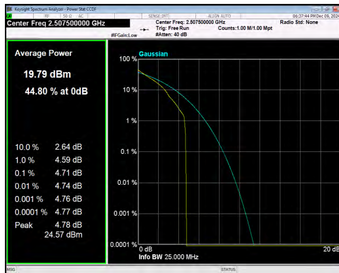
Band7 QPSK BW=15MHz Channel=21100 RB Size=1 Position=#0
