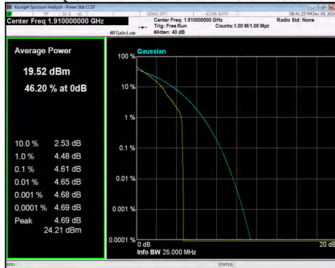
Band25 QPSK BW=15MHz Channel=26115 RB Size=1 Position=#0
