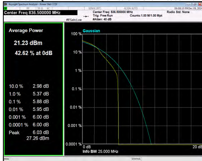
Band5 16QAM BW=10MHz Channel=20600 RB Size=1 Position=#0
