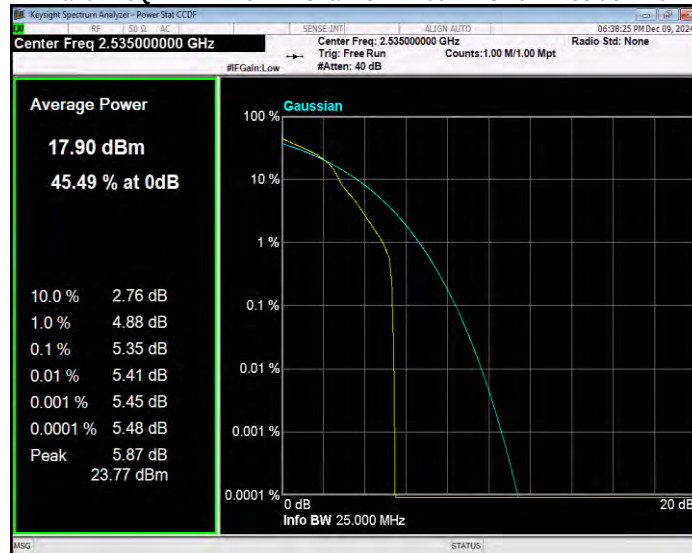
Band7 16QAM BW=20MHz Channel=21350 RB Size=1 Position=#0
