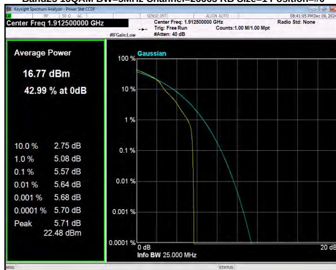
Band25 16QAM BW=5MHz Channel=26665 RB Size=1 Position=#0
