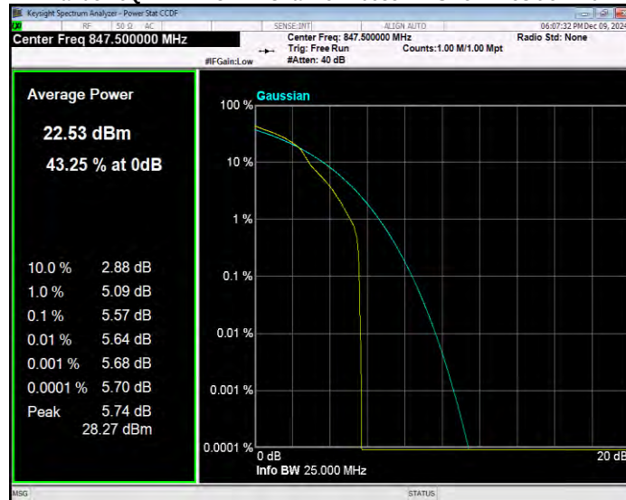
Band5 16QAM BW=3MHz Channel=20525 RB Size=1 Position=#0
