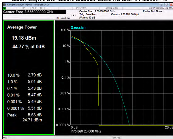
Band7 16QAM BW=15MHz Channel=21375 RB Size=1 Position=#0
