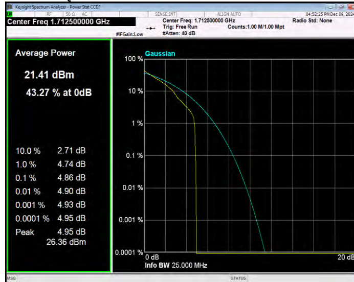
Band5 16QAM BW=1.4MHz Channel=20407 RB Size=1 Position=#0
