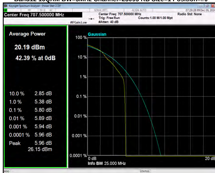
Band12 16QAM BW=5MHz Channel=23155 RB Size=1 Position=#0
