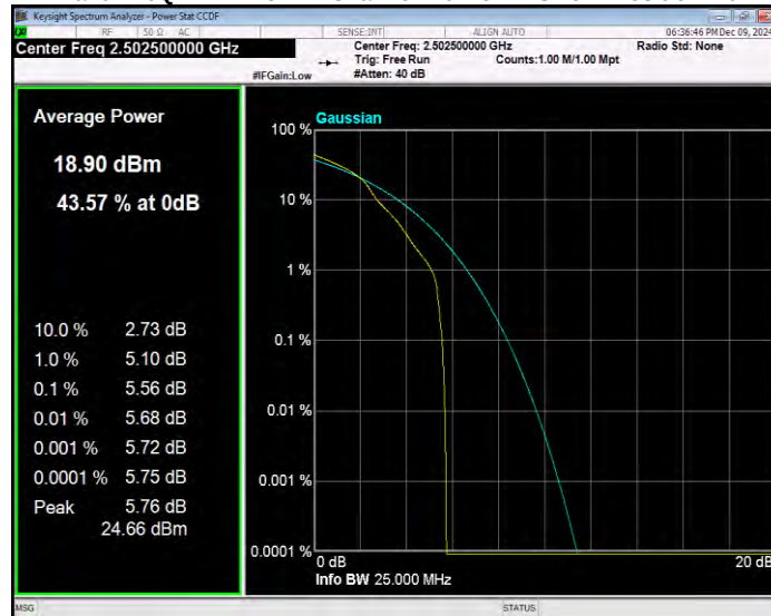
Band7 16QAM BW=5MHz Channel=21425 RB Size=1 Position=#0
