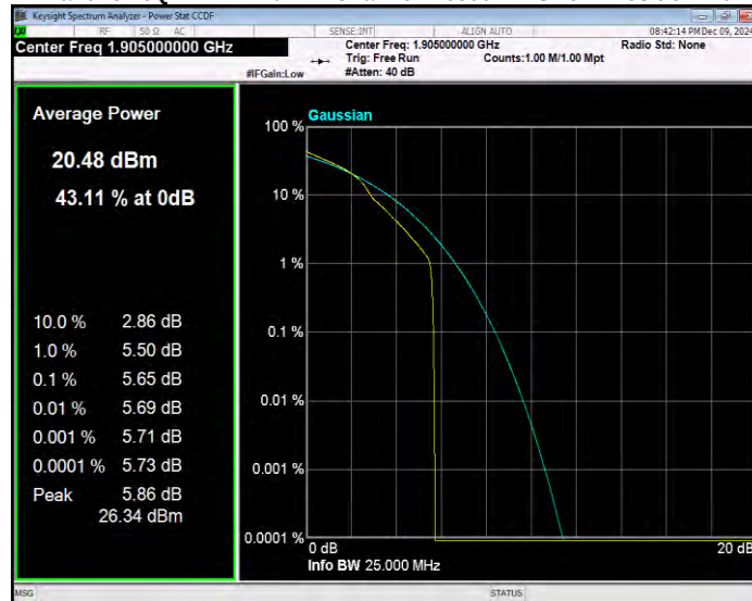
Band25 QPSK BW=1.4MHz Channel=26047 RB Size=1 Position=#0
