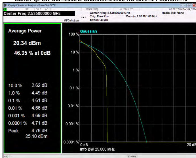
Band7 QPSK BW=10MHz Channel=21400 RB Size=1 Position=#0
