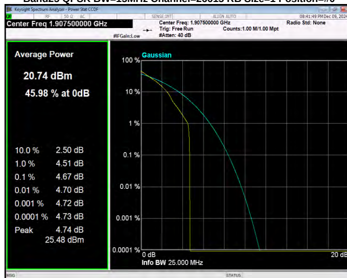
Band25 QPSK BW=5MHz Channel=26065 RB Size=1 Position=#0
