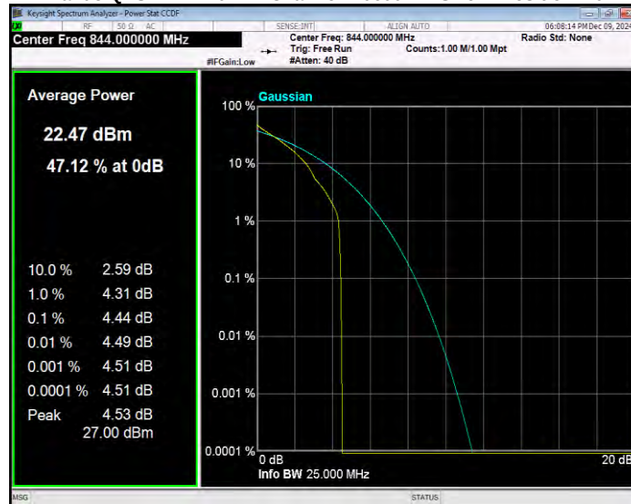
Band5 QPSK BW=5MHz Channel=20525 RB Size=1 Position=#0
