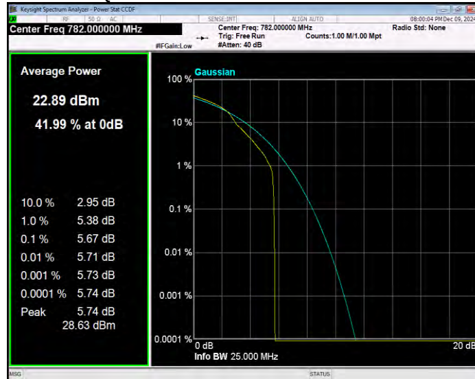
Band13 16QAM BW=5MHz Channel=23255 RB Size=1 Position=#0
