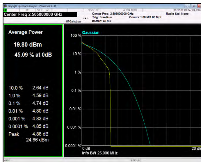
Band7 QPSK BW=10MHz Channel=21100 RB Size=1 Position=#0
