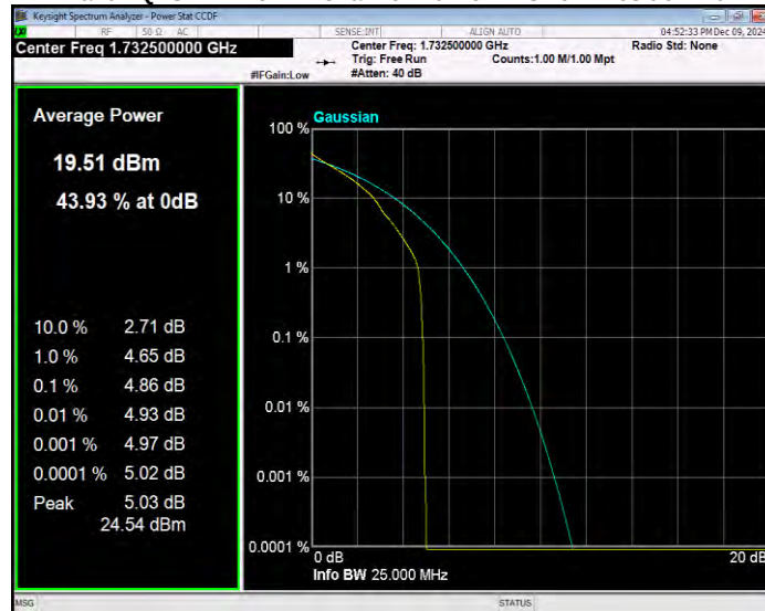
Band4 QPSK BW=5MHz Channel=19975 RB Size=1 Position=#0
