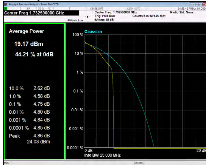
Band4 QPSK BW=20MHz Channel=20300 RB Size=1 Position=#0
