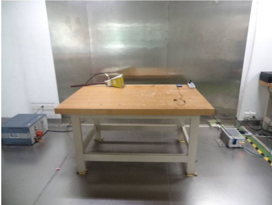
Conducted Emissions - Front View
