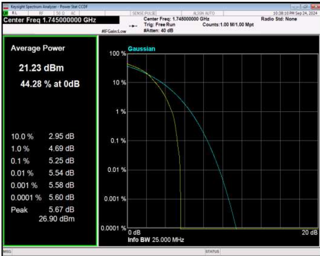
Band66 QPSK BW=15MHz Channel=132322 RB Size=1 Position=#0
