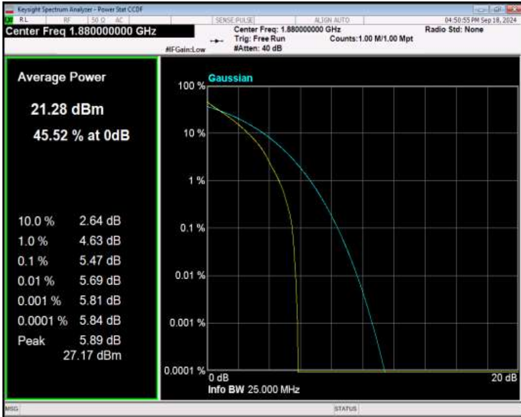
Band2 16QAM BW=3MHz Channel=18900 RB Size=1 Position=#0
