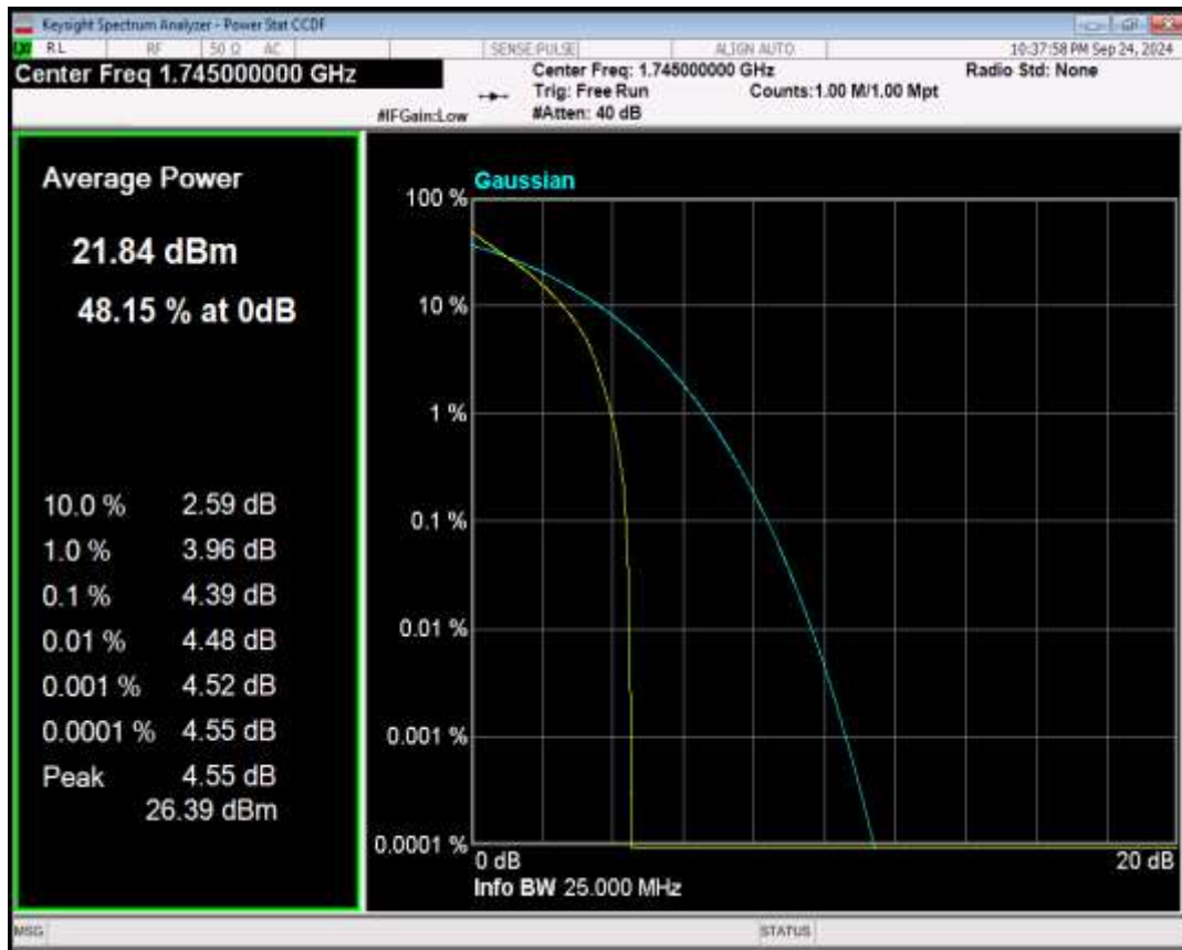
Band66 16QAM BW=3MHz Channel=132322 RB Size=1 Position=#0
