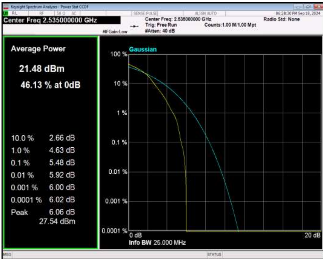
Band7 QPSK BW=20MHz Channel=21100 RB Size=1 Position=#0
