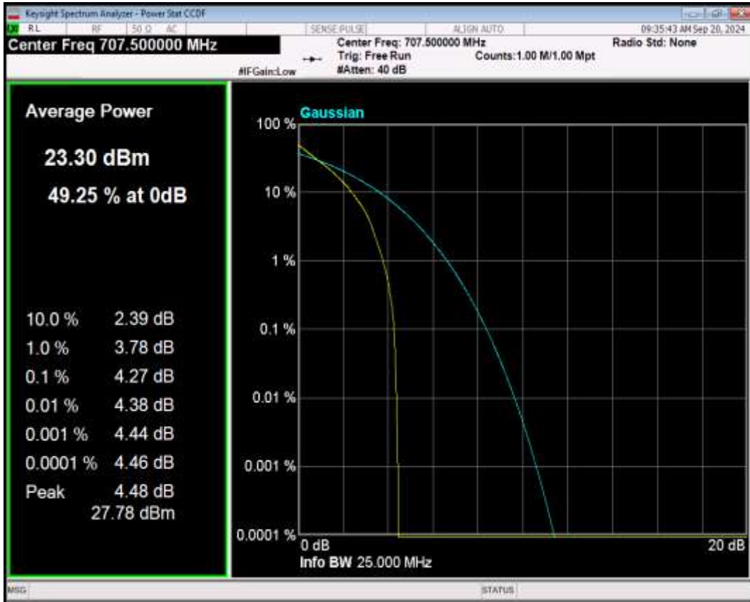
Band12 16QAM BW=10MHz Channel=23095 RB Size=1 Position=#0
