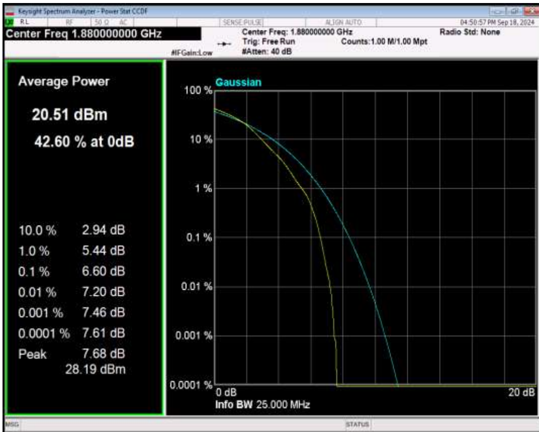
Band2 QPSK BW=5MHz Channel=18900 RB Size=1 Position=#0
