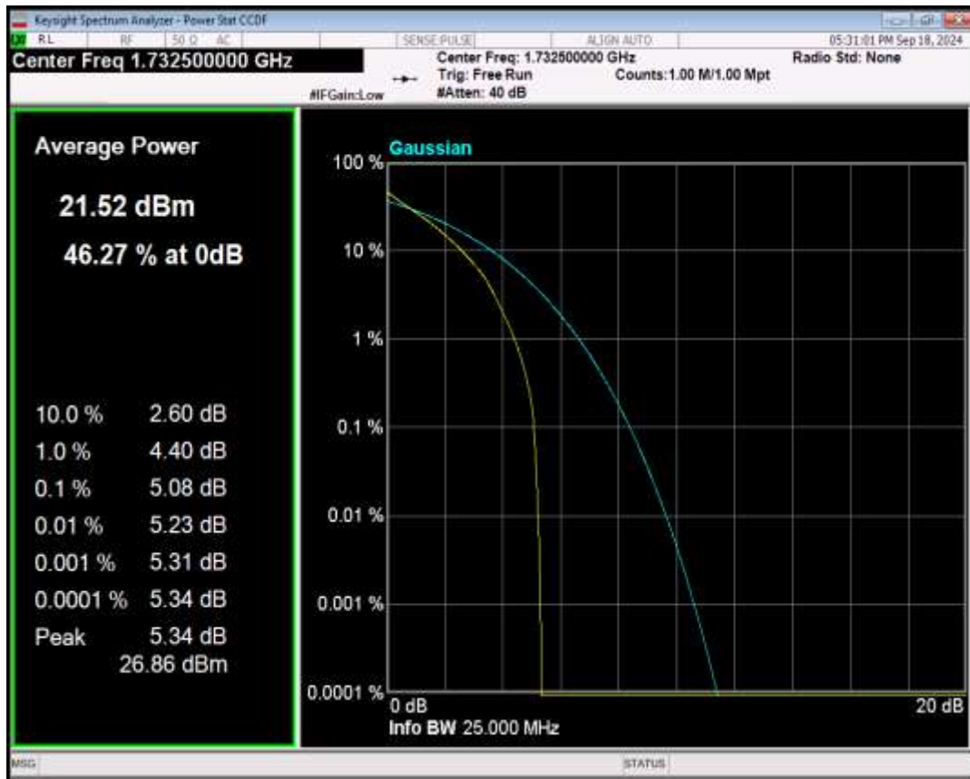
Band4 16QAM BW=15MHz Channel=20175 RB Size=1 Position=#0
