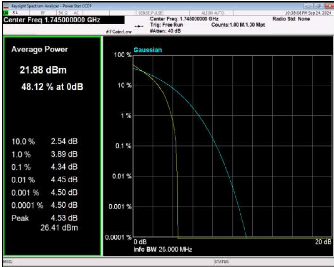
Band66 16QAM BW=10MHz Channel=132322 RB Size=1 Position=#0
