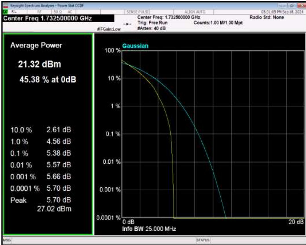
Band4 16QAM BW=20MHz Channel=20175 RB Size=1 Position=#0
