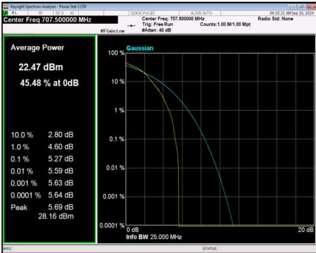
Band12 QPSK BW=3MHz Channel=23095 RB Size=1 Position=#0
