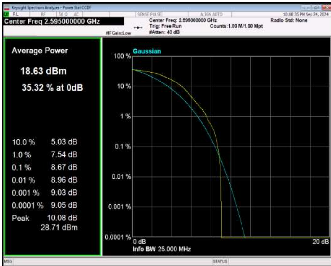
Band41 QPSK BW=10MHz Channel=40640 RB Size=1 Position=#0
