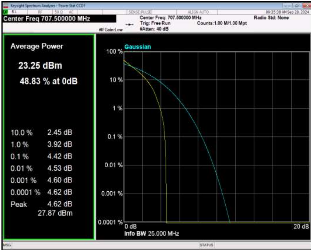
Band12 16QAM BW=5MHz Channel=23095 RB Size=1 Position=#0
