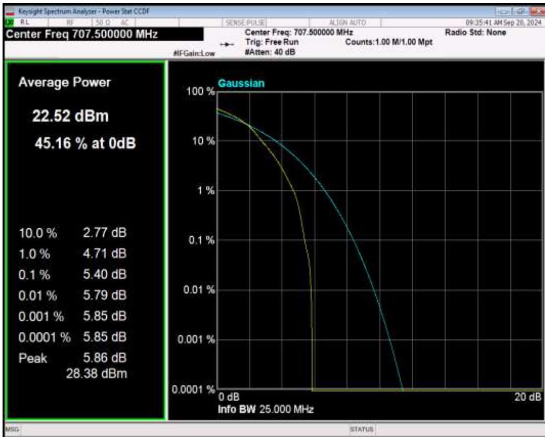
Band12 QPSK BW=10MHz Channel=23095 RB Size=1 Position=#0
