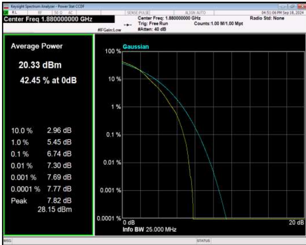
Band2 QPSK BW=15MHz Channel=18900 RB Size=1 Position=#0
