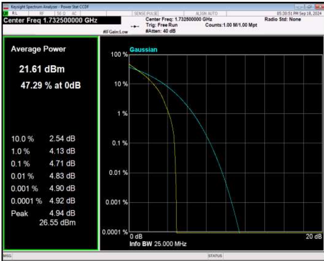
Band4 16QAM BW=5MHz Channel=20175 RB Size=1 Position=#0
