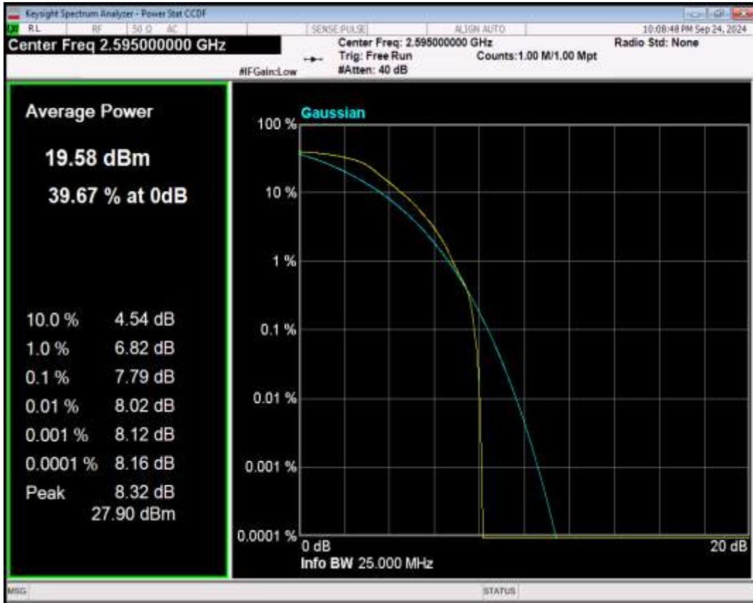
Band41 16QAM BW=20MHz Channel=40640 RB Size=1 Position=#0
