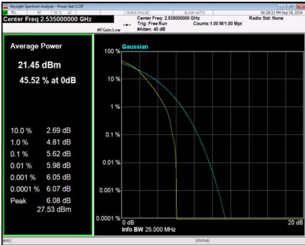
Band7 QPSK BW=10MHz Channel=21100 RB Size=1 Position=#0
