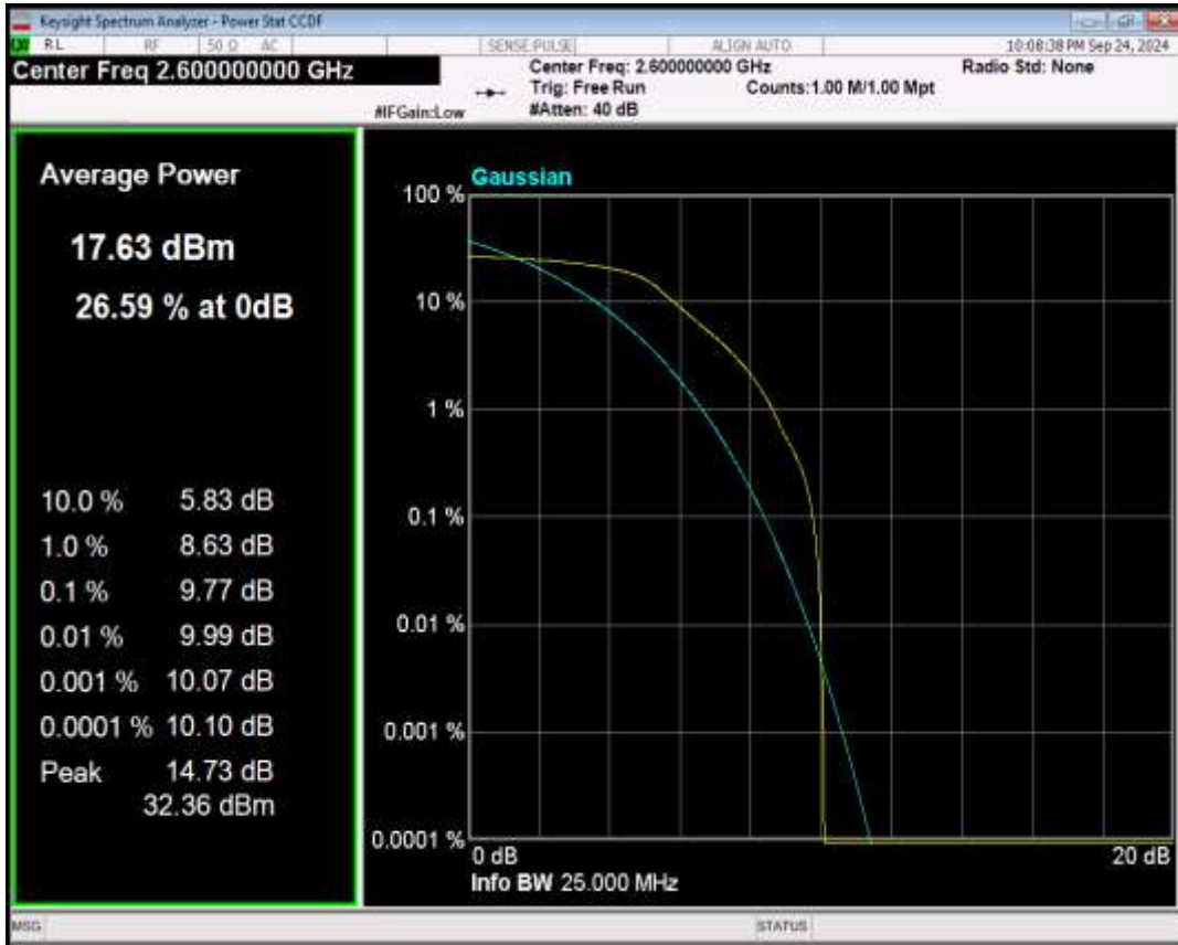
Band41 16QAM BW=10MHz Channel=40640 RB Size=1 Position=#0
