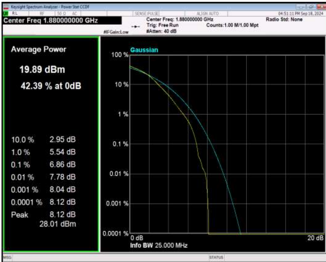
Band2 QPSK BW=20MHz Channel=18900 RB Size=1 Position=#0
