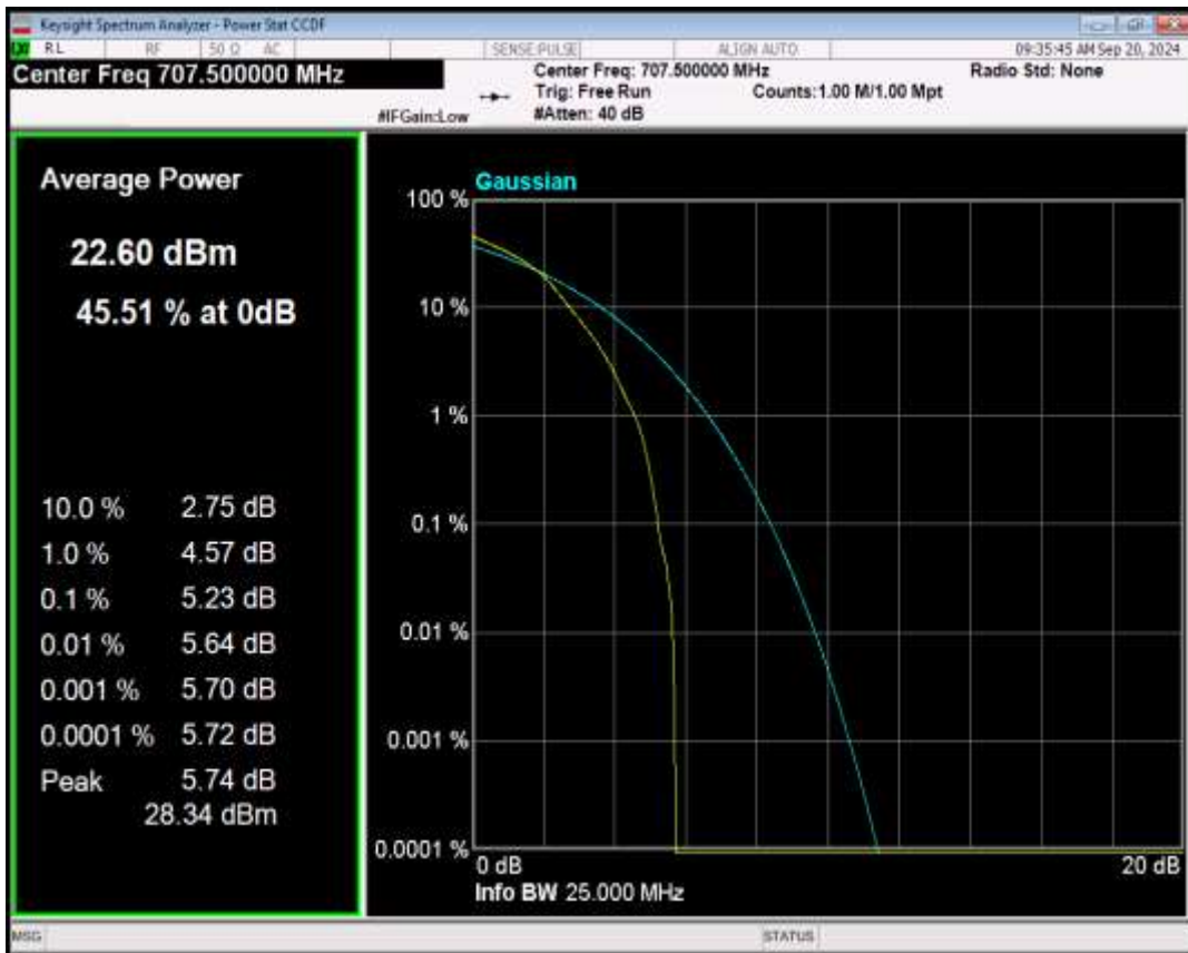
Band17 QPSK BW=5MHz Channel=23790 RB Size=1 Position=#0
