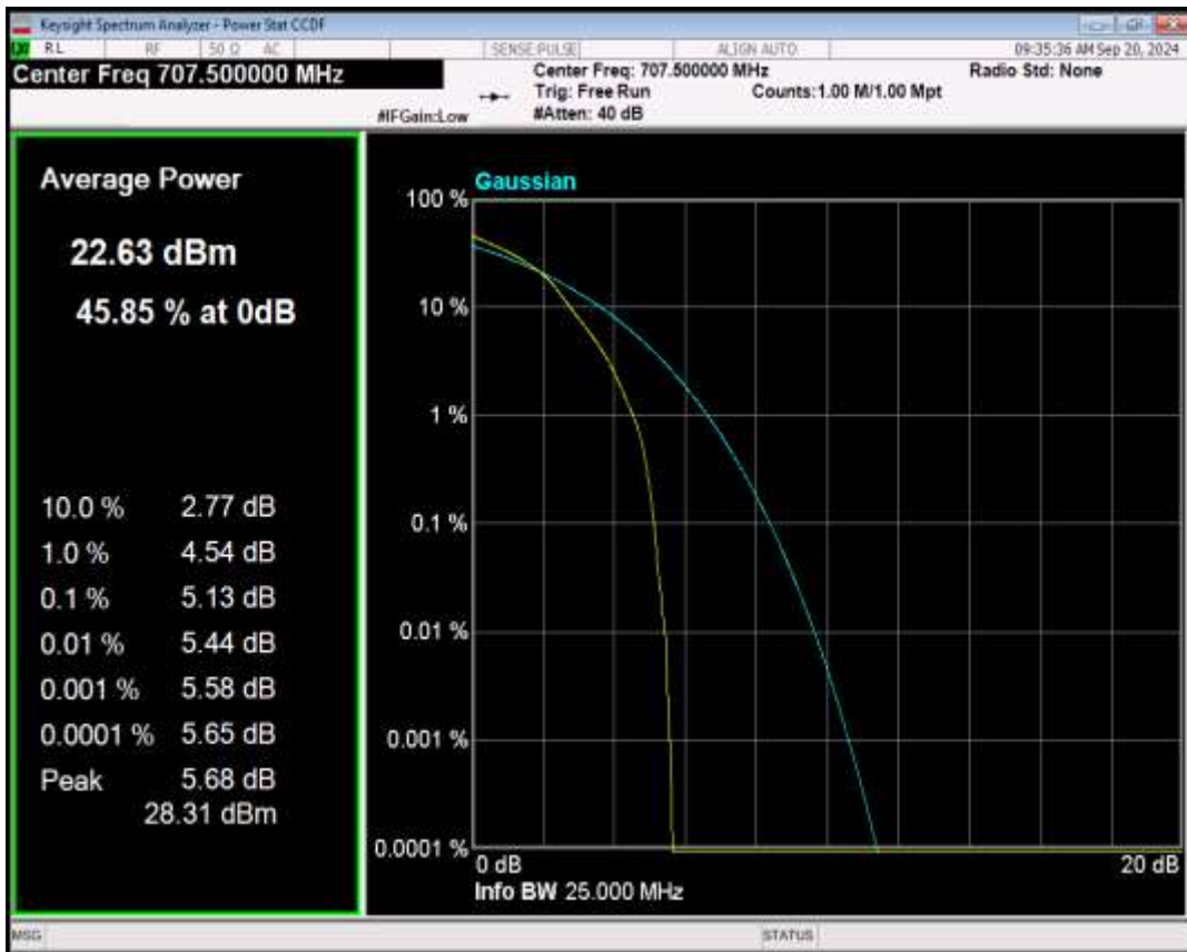
Band12 QPSK BW=5MHz Channel=23095 RB Size=1 Position=#0
