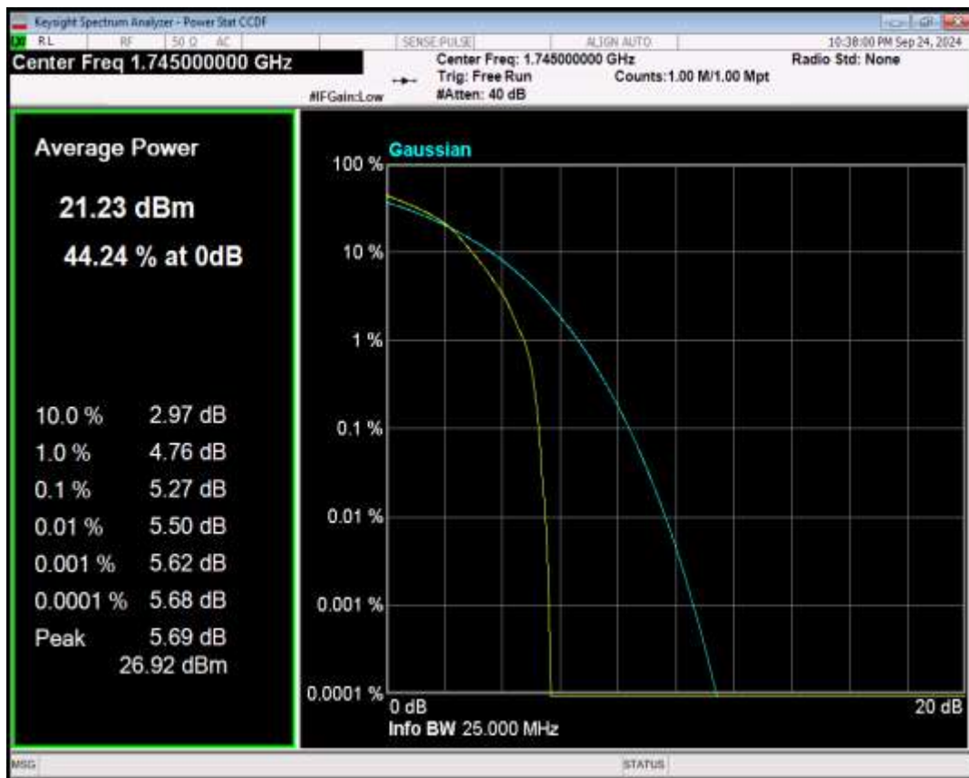
Band66 QPSK BW=5MHz Channel=132322 RB Size=1 Position=#0
