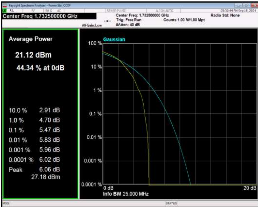
Band4 QPSK BW=5MHz Channel=20175 RB Size=1 Position=#0
