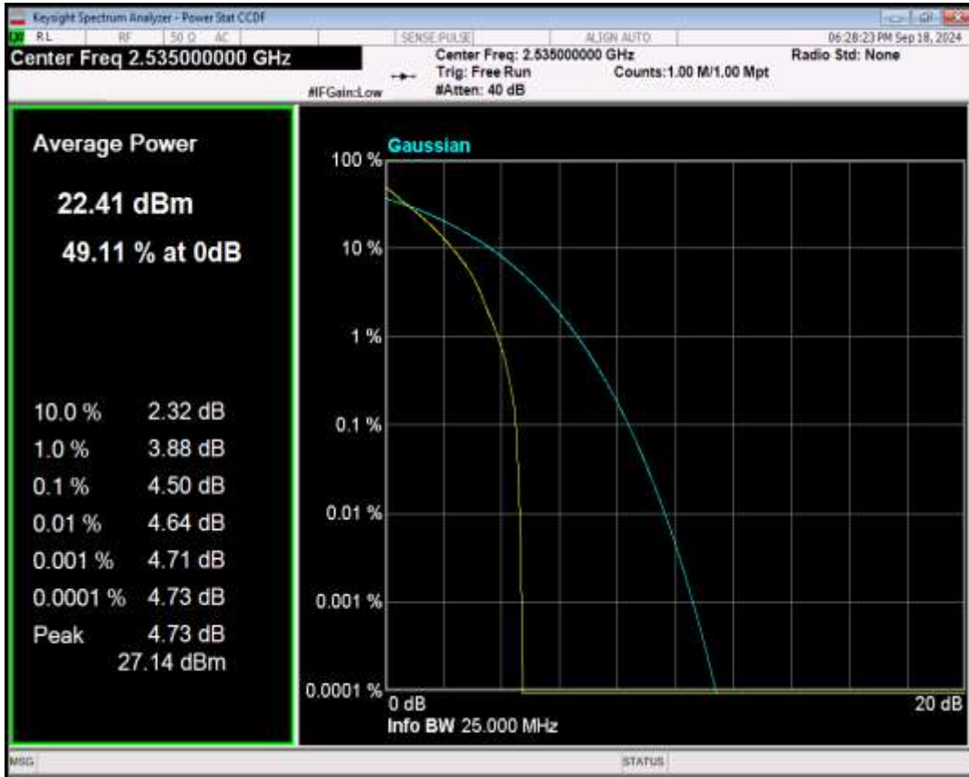
Band7 16QAM BW=10MHz Channel=21100 RB Size=1 Position=#0
