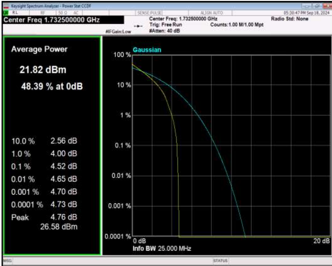
Band4 16QAM BW=3MHz Channel=20175 RB Size=1 Position=#0
