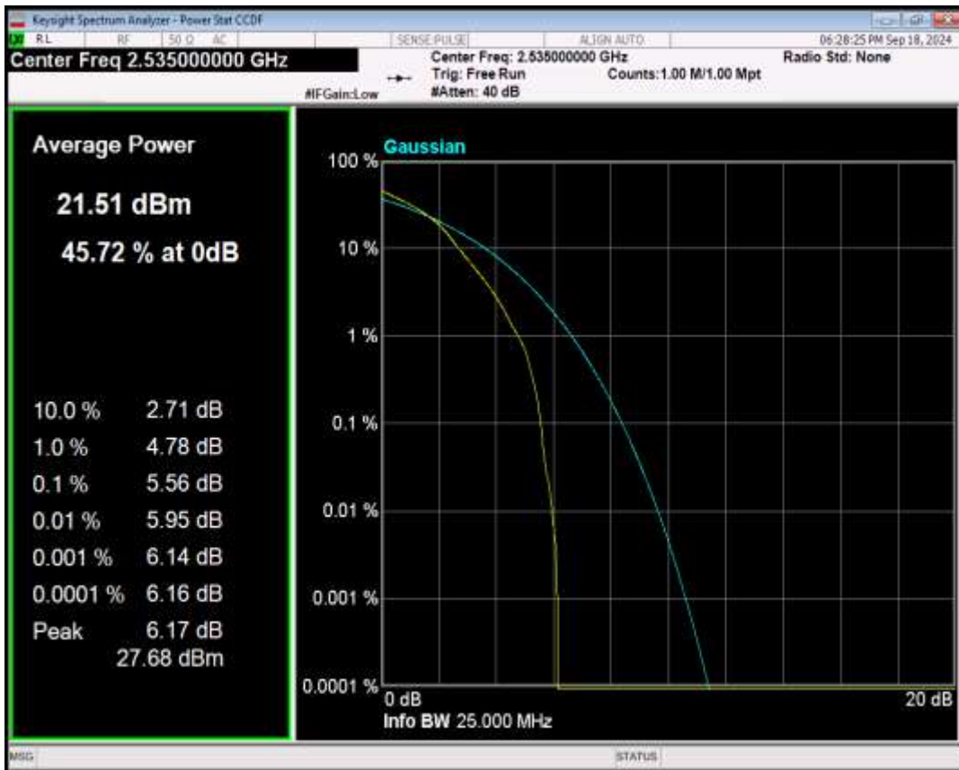
Band7 QPSK BW=15MHz Channel=21100 RB Size=1 Position=#0
