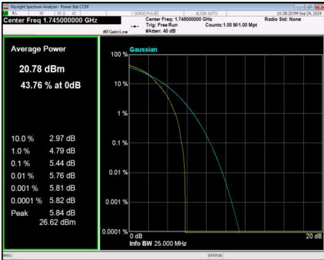
Band7 QPSK BW=5MHz Channel=21100 RB Size=1 Position=#0
