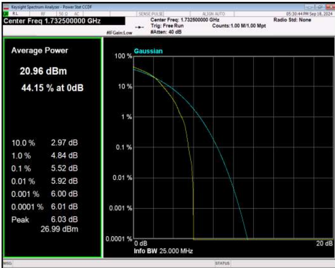
Band4 QPSK BW=3MHz Channel=20175 RB Size=1 Position=#0
