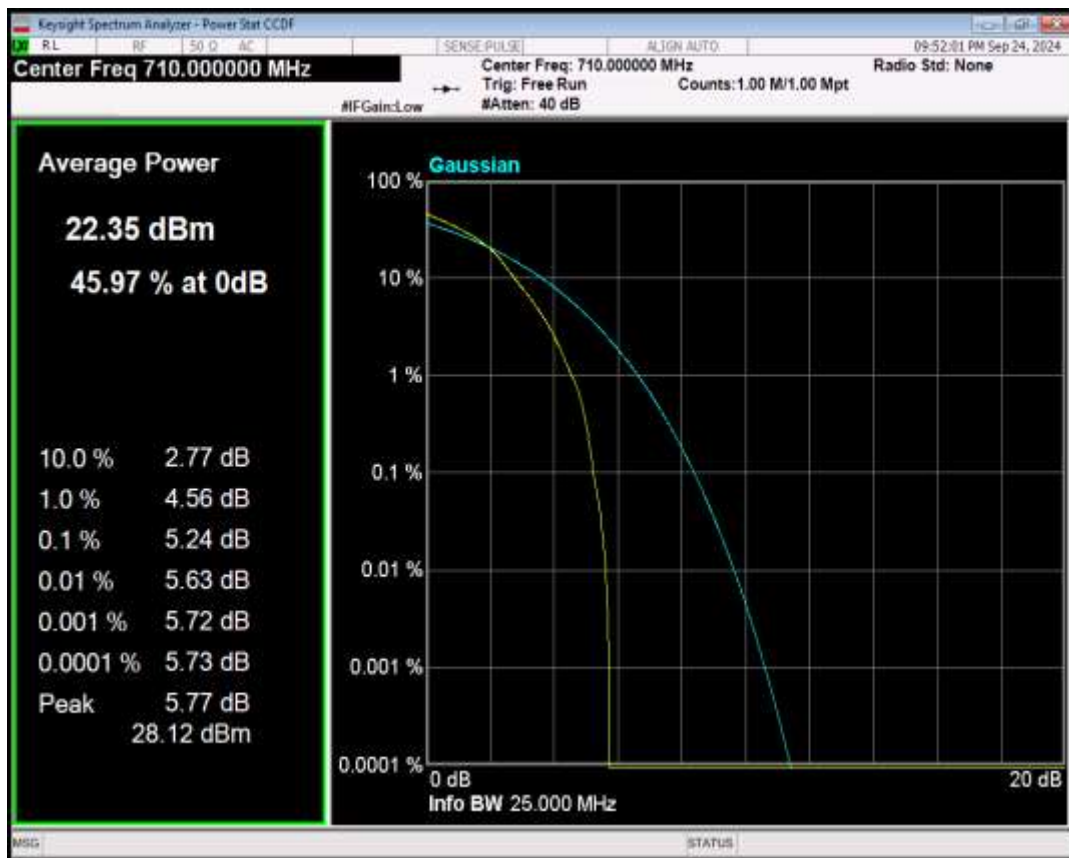
Band17 QPSK BW=10MHz Channel=23790 RB Size=1 Position=#0
