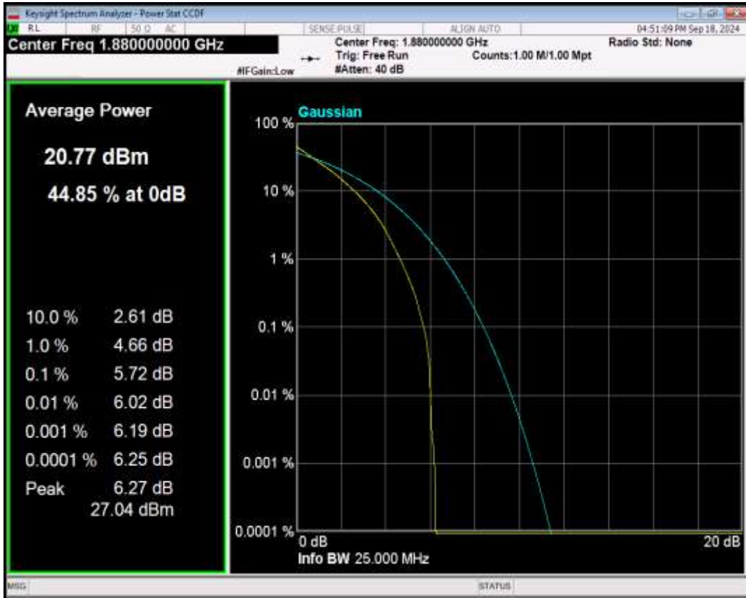
Band2 16QAM BW=15MHz Channel=18900 RB Size=1 Position=#0
