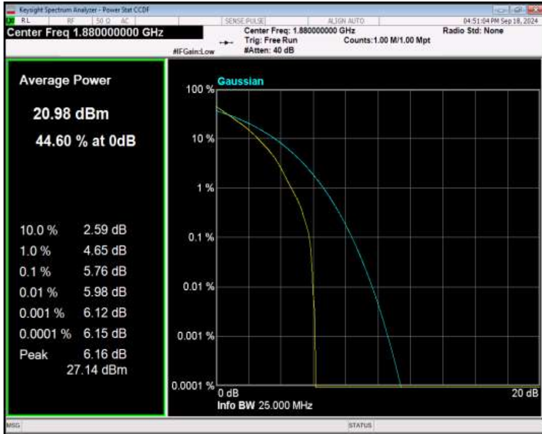
Band2 16QAM BW=10MHz Channel=18900 RB Size=1 Position=#0
