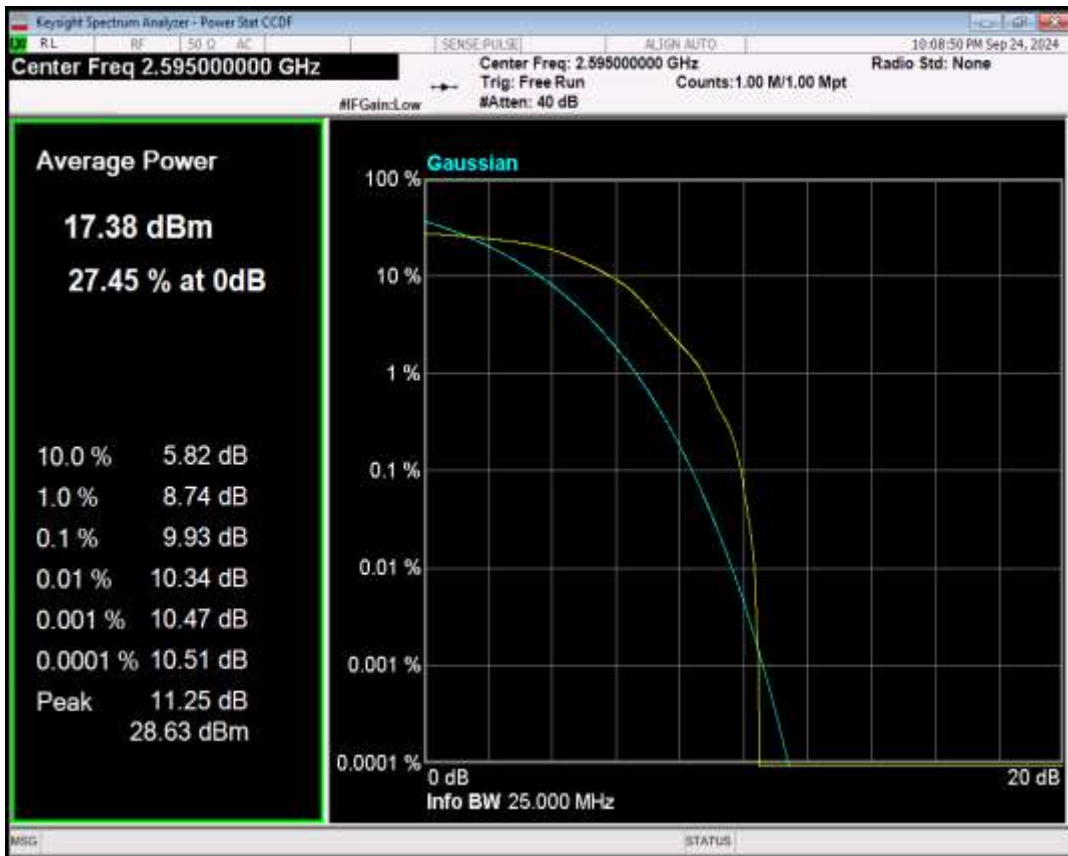
Band5 QPSK BW=1.4MHz Channel=20525 RB Size=1 Position=#0
