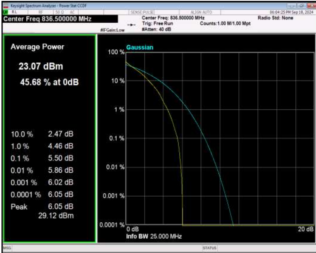
Band5 16QAM BW=10MHz Channel=20525 RB Size=1 Position=#0
