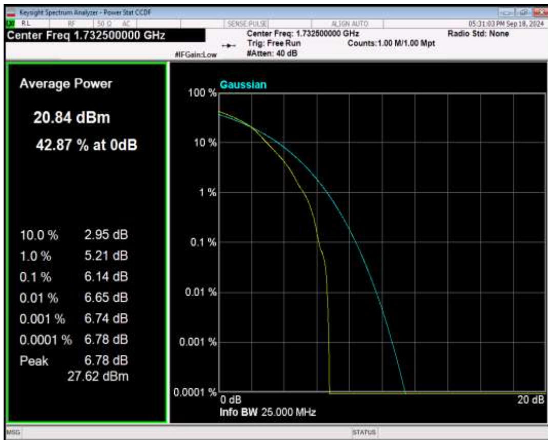
Band4 QPSK BW=20MHz Channel=20175 RB Size=1 Position=#0
