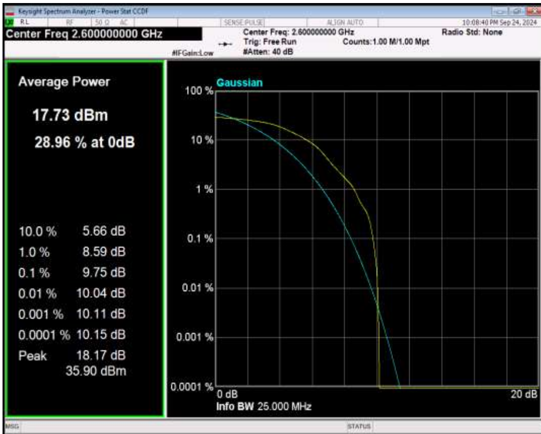
Band41 QPSK BW=15MHz Channel=40640 RB Size=1 Position=#0
