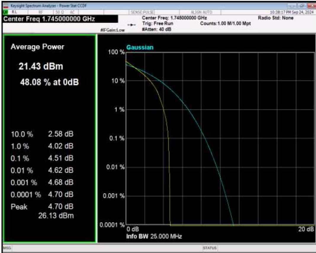
Band66 16QAM BW=20MHz Channel=132322 RB Size=1 Position=#0
