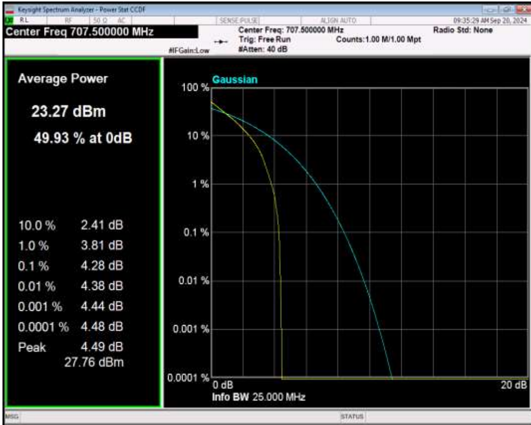
Band12 16QAM BW=1.4MHz Channel=23095 RB Size=1 Position=#0
