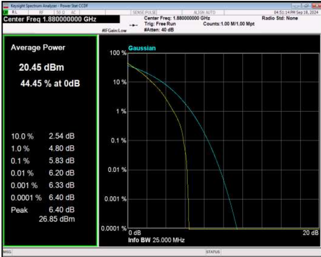
Band2 16QAM BW=20MHz Channel=18900 RB Size=1 Position=#0
