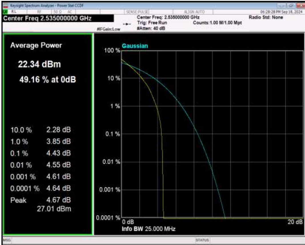
Band7 16QAM BW=15MHz Channel=21100 RB Size=1 Position=#0
