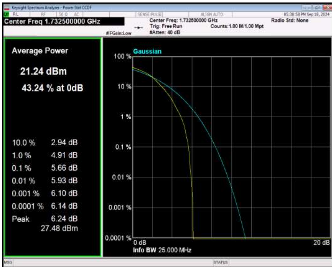
Band4 QPSK BW=15MHz Channel=20175 RB Size=1 Position=#0
