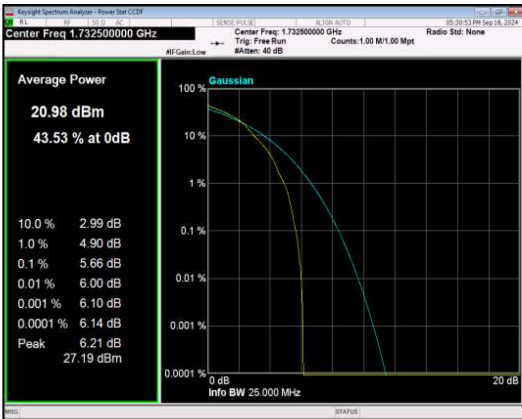
Band4 QPSK BW=10MHz Channel=20175 RB Size=1 Position=#0
