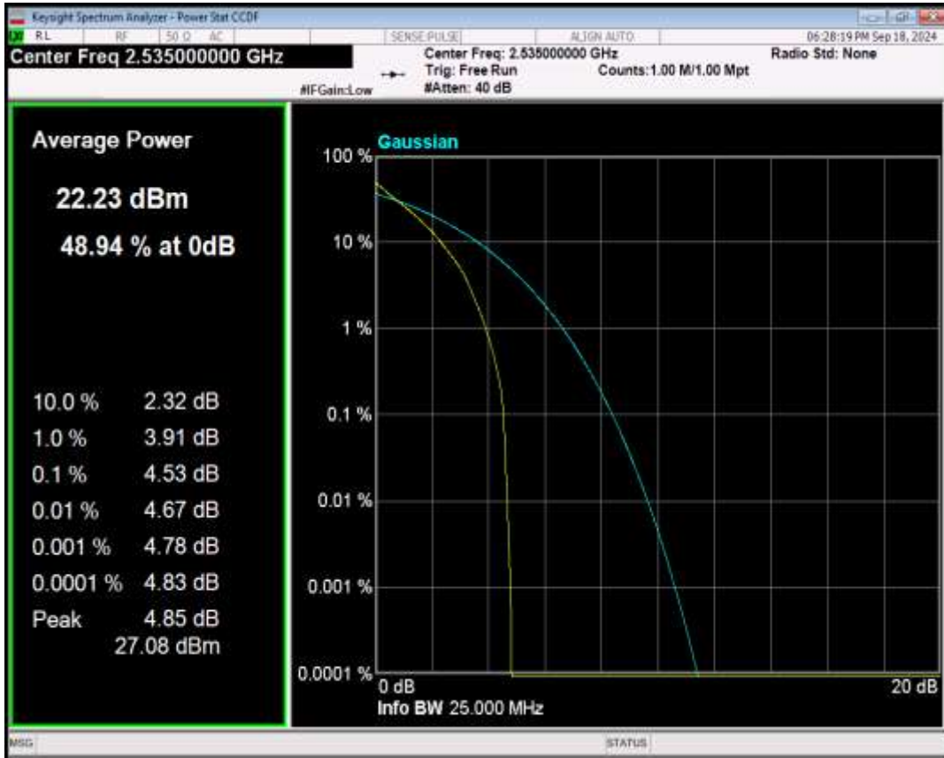
Band7 16QAM BW=5MHz Channel=21100 RB Size=1 Position=#0
