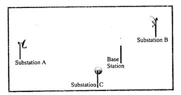
In this example, the base station communicates directly with each substation. The substations communicate with each other through the base station.
