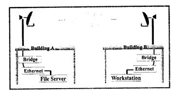
In this configuration the LAN in Building A is connected to the LAN in Building B only by the wireless link, and the only packets sent between the two LAN systems are packets specifically destined from one LAN to the other. The MP1100E supports both point-to-point and multi-point wireless connections.
