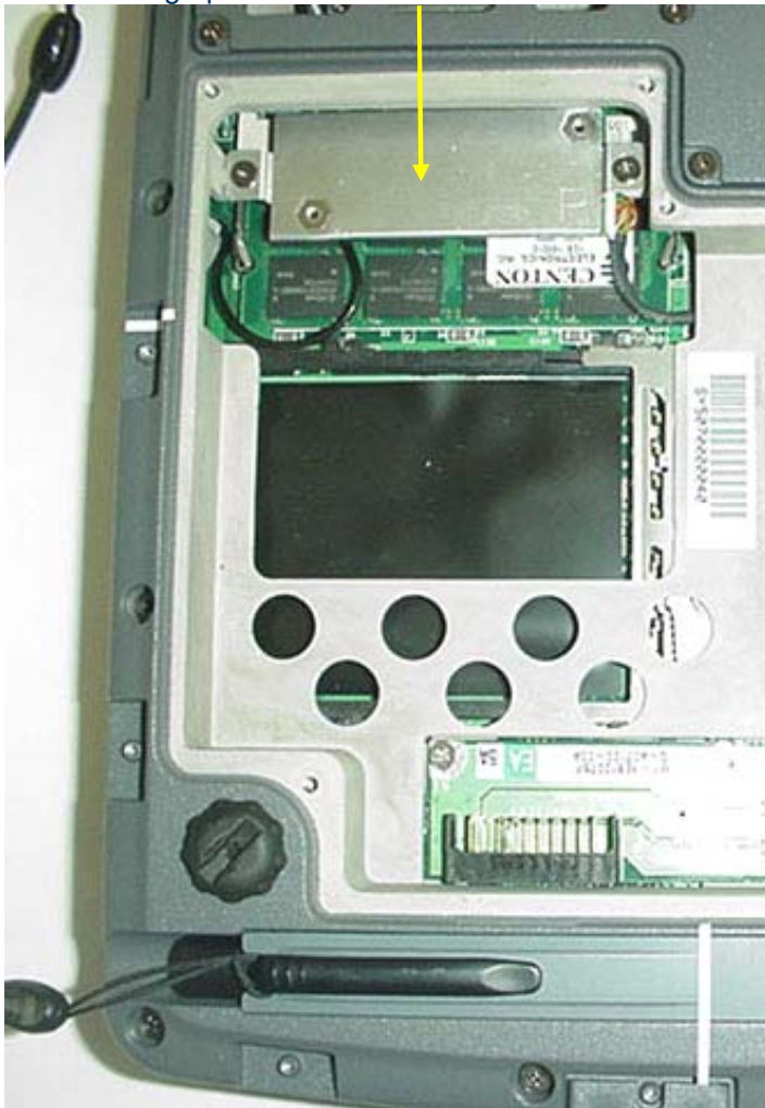
Photograph A.1-5 - Internal Bluetooth Location
