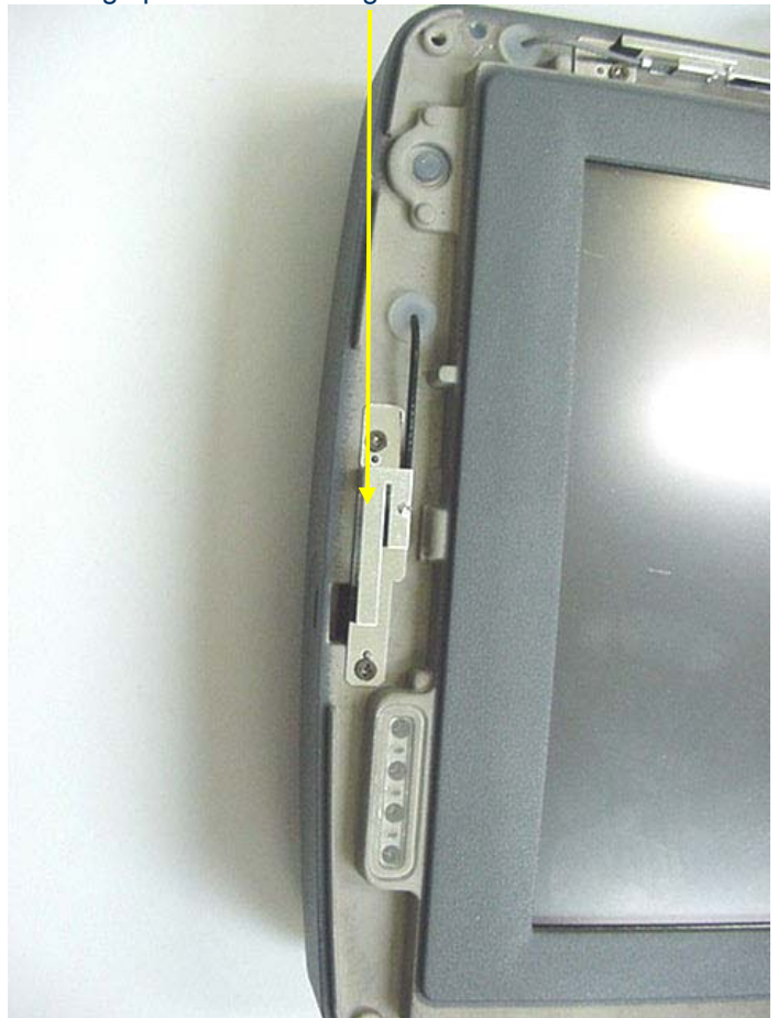
Photograph A.1-6 - Left Edge Bluetooth Antenna Location
