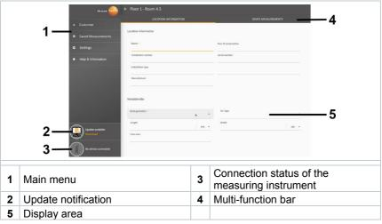
Operation of the software is based on the same functional principle as the instrument firmware for the testo 400.
