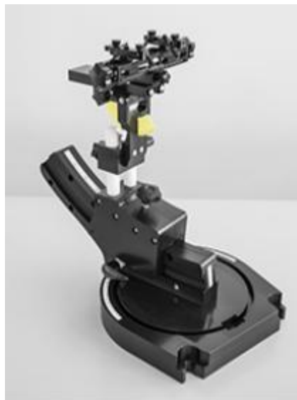
Device holder supplied by SPEAG
