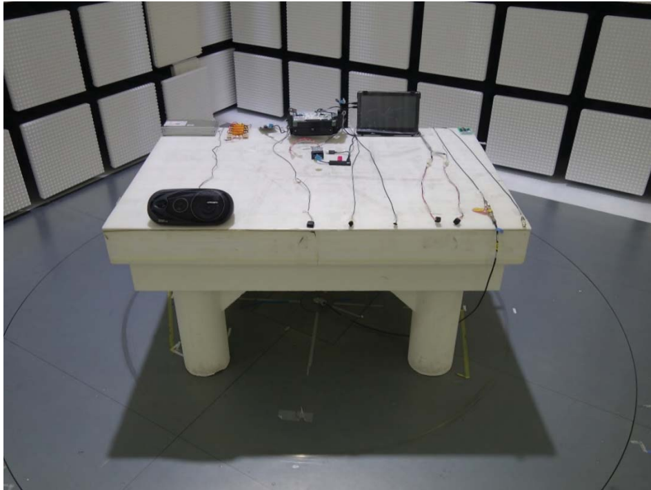
Photograph 1: Set-up for Radiated Emission, Front View
