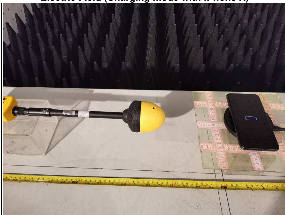
Electric Field (Charging mode with iPhone X)
