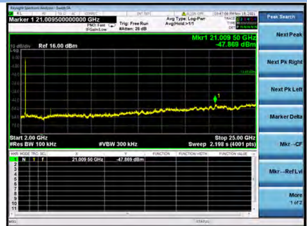
802.11b 11 CHANNEL, SPURIOUS 2 GHz ~ 25 GHz
