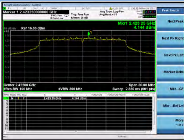
802.11n-20 MHz 3 CHANNEL, Carrier level
