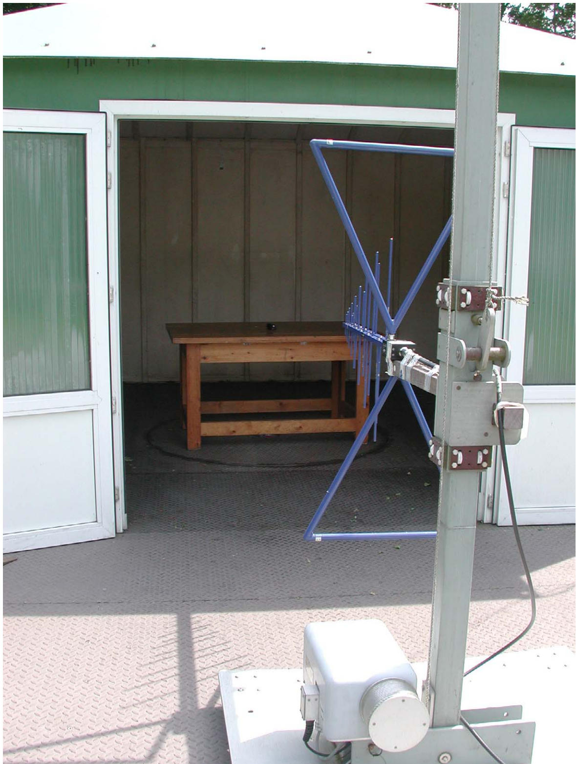
Photograph 15: Test setup OATS > 30 MHz
