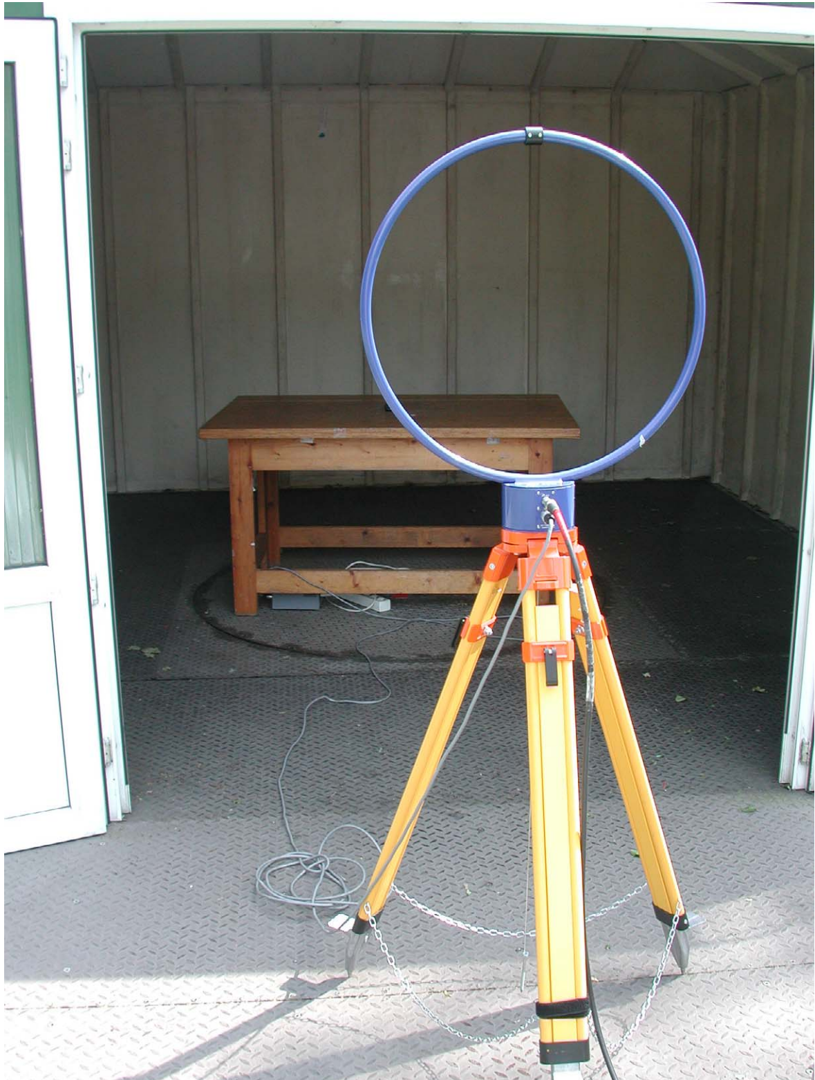
Photograph 14: Test setup OATS < 30 MHz
