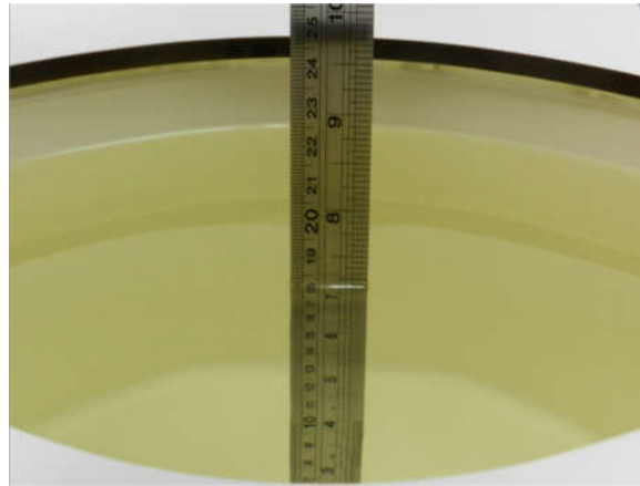
Fig 10.2 Photo of Liquid Height for Body SAR
