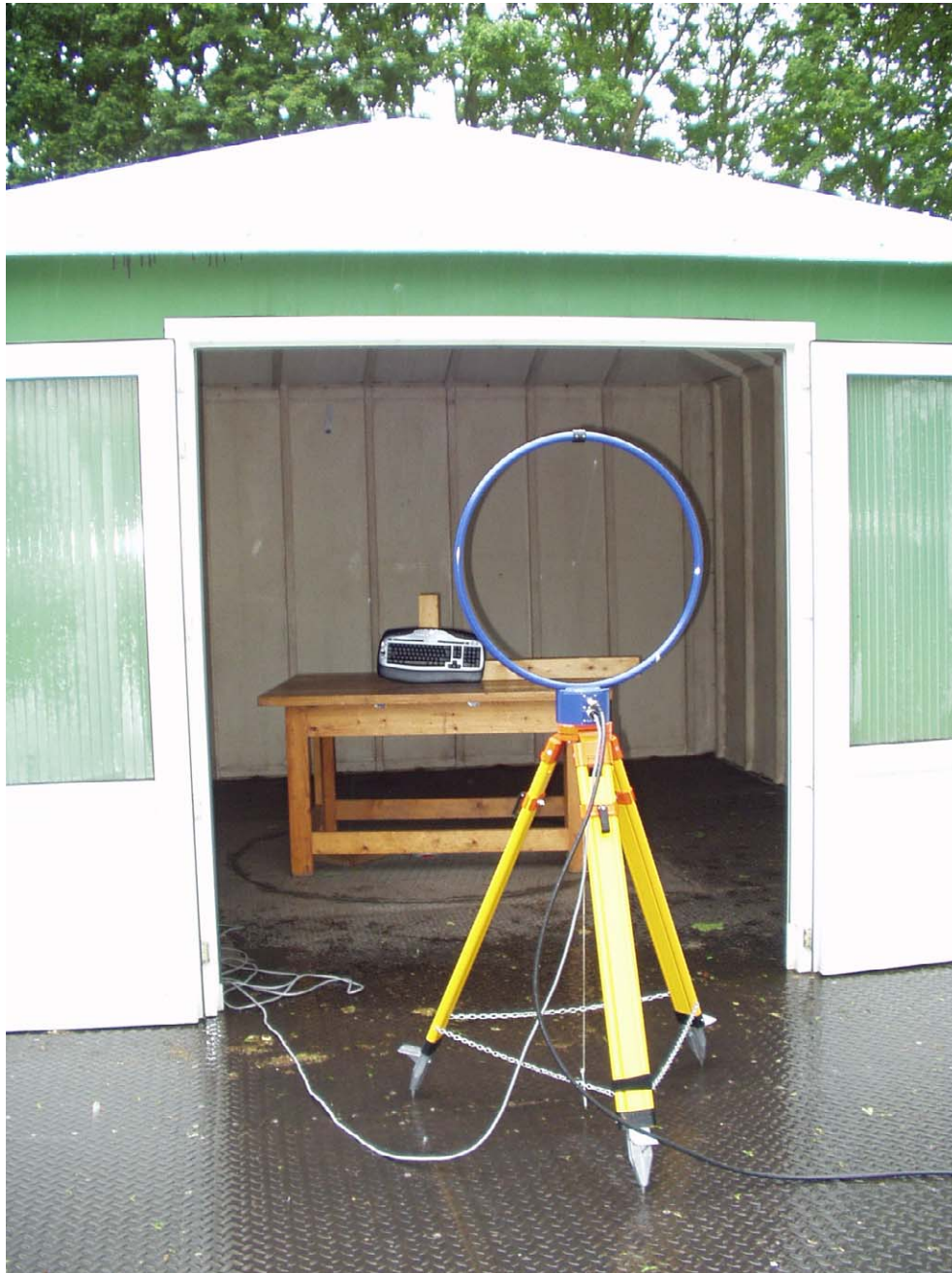
Photograph 7: Test setup OATS < 30 MHz
