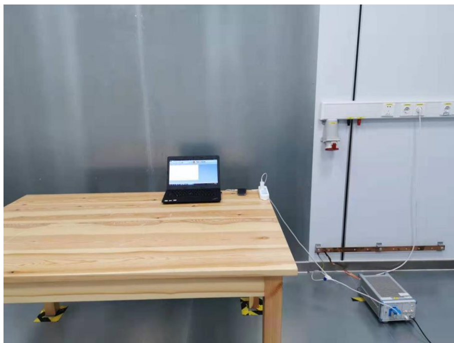
Fig. 4 Power line conducted emission setup photo
