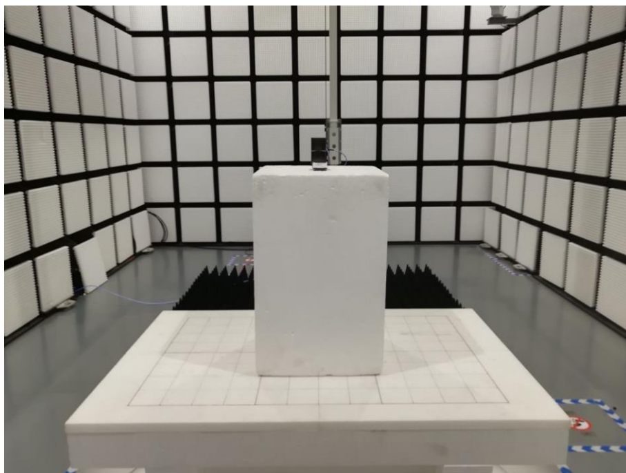
Fig. 3 Radiated emission setup photo(Above 1GHz)
