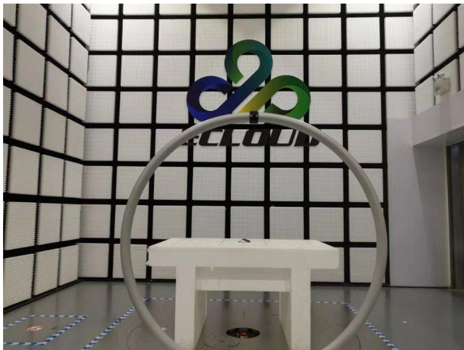
Fig. 1 Radiated emission setup photo(Below 30MHz)
