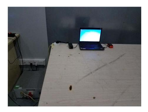
Radiation Emission Test Setup (30MHz to 1GHz)
