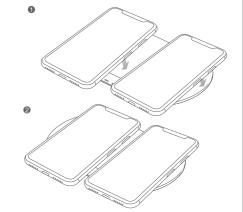
Make sure the wireless charger dock connect to the power supply. ② Put the Oi-enabled smart phone properly on the transmitter, the indicator light become blue and start charging. The device enter to standby mode when take away the phone from charging pad.
