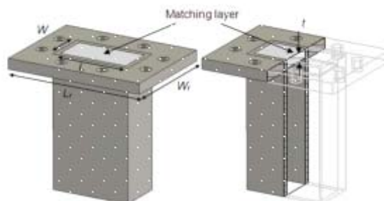
Figure 1: Validation Waveguide Dimensions
