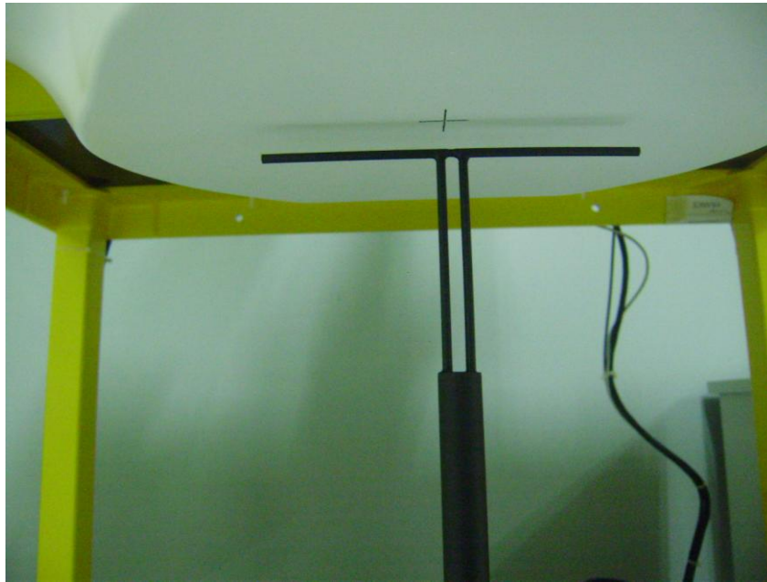
Setup Photo of Dipole Antenna
