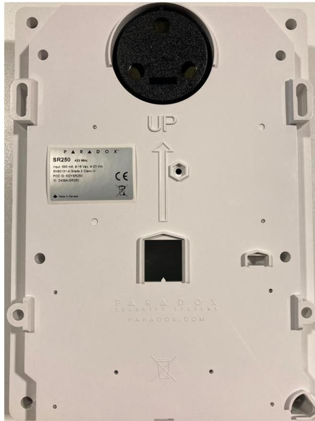
Label with **FCC ID: KDYSR250** and **IC: 2438A-SR250** will be located here. The statement according to FCC part 15 §15.19(a)(3) is placed in User Manual, page ... (Application exhibit User\_manual\_36712).
