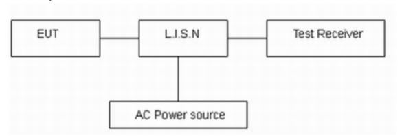
Note: AC Power source is used to change the voltage 120V/60Hz.
