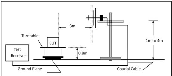
(c) For radiated emissions above 1000MHz
