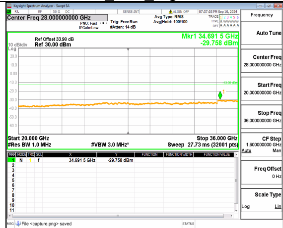
n77(3450-3550MHz) (20GHz-36GHz) 60M DFT-s-OFDM BPSK Inner_1RB_Left High
