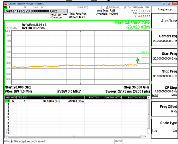
n77(3450-3550MHz) (20GHz-36GHz) 60M DFT-s-OFDM QPSK Inner_1RB_Left Mid
