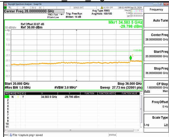
n77(3450-3550MHz) (20GHz-36GHz) 80M DFT-s-OFDM QPSK Inner_1RB_Left Low
