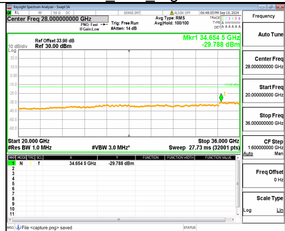
n77(3450-3550MHz) (20GHz-36GHz) 30M DFT-s-OFDM BPSK Inner_1RB_Left High
