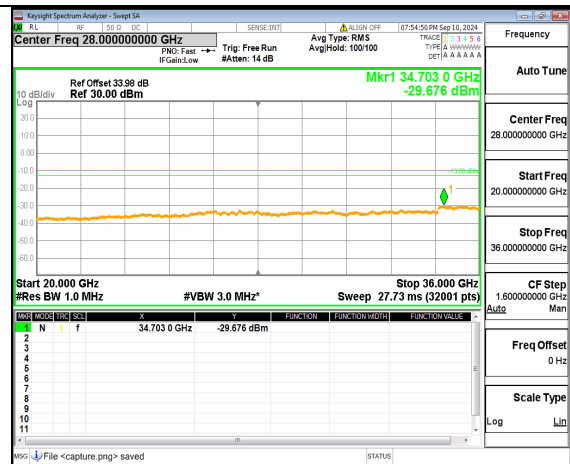
n77(3450-3550MHz) (20GHz-36GHz) 70M DFT-s-OFDM BPSK Inner_1RB_Right High
