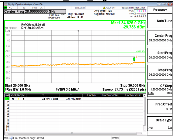
n77(3450-3550MHz) (20GHz-36GHz) 40M DFT-s-OFDM BPSK Inner_1RB_Left Mid
