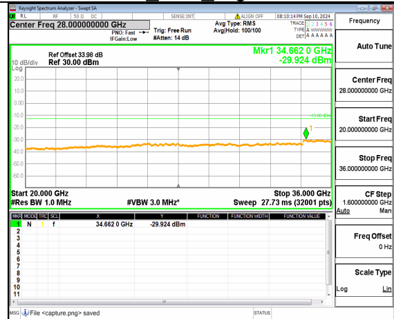
n77(3450-3550MHz) (20GHz-36GHz) 80M DFT-s-OFDM BPSK Inner_1RB_Left High
