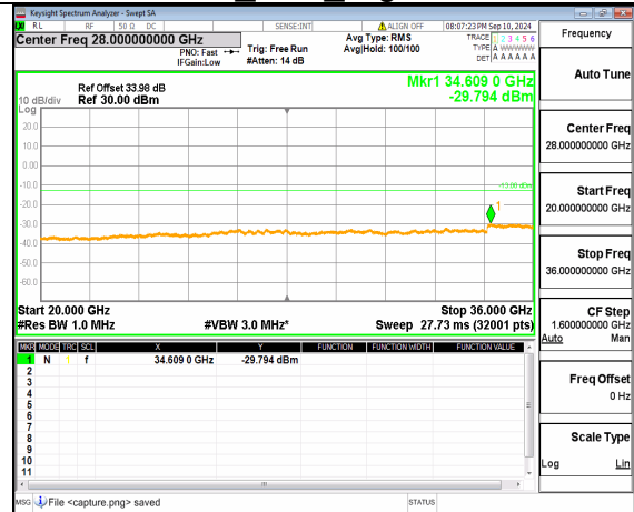
n77(3450-3550MHz) (20GHz-36GHz) 80M DFT-s-OFDM QPSK Inner_1RB_Left Mid
