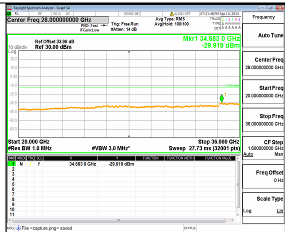
n77(3450-3550MHz) (20GHz-36GHz) 50M DFT-s-OFDM BPSK Inner_1RB_Right High
