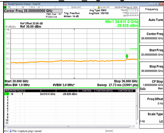
n77(3450-3550MHz) (20GHz-36GHz) 30M DFT-s-OFDM QPSK Inner_1RB_Left High
