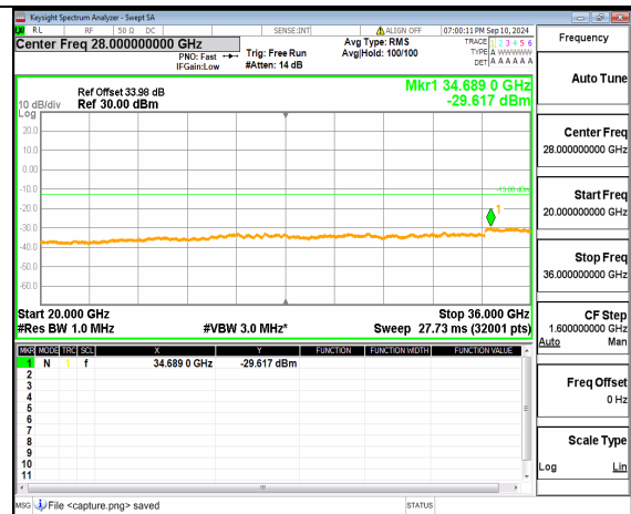
n77(3450-3550MHz) (20GHz-36GHz) 40M DFT-s-OFDM BPSK Inner_1RB_Right Mid
