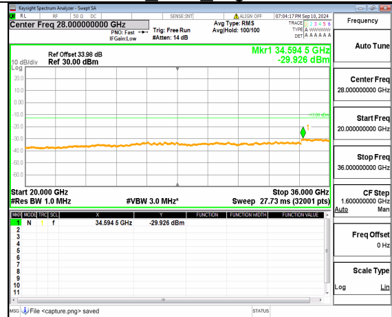
n77(3450-3550MHz) (20GHz-36GHz) 40M DFT-s-OFDM BPSK Inner_1RB_Left High
