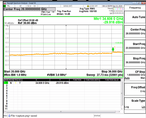
n77(3450-3550MHz) (20GHz-36GHz) 80M DFT-s-OFDM QPSK Inner_1RB_Left High
