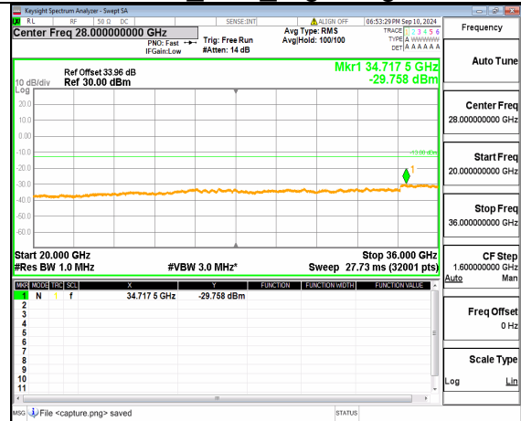
n77(3450-3550MHz) (20GHz-36GHz) 40M DFT-s-OFDM BPSK Inner_1RB_Left Low
