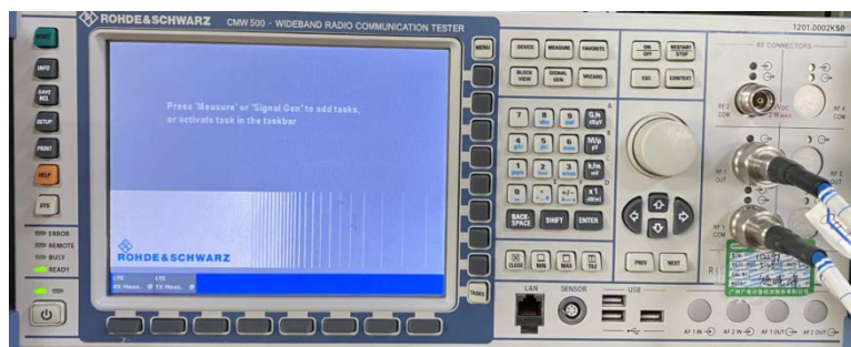
CMW 500 (2G/3G/4G Test Equipment)
