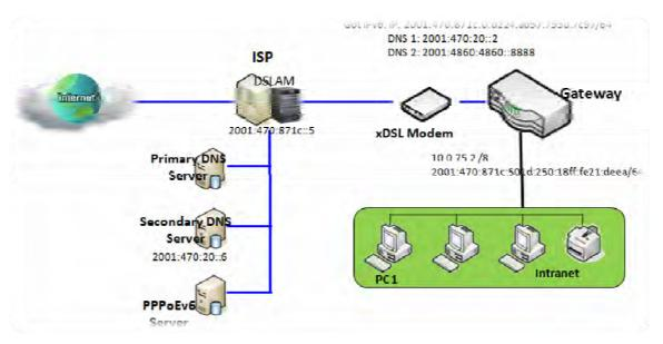
The diagram above depicts the IPv6 addressing through PPPoE, PPPoEv6 server (DSLAM) on the ISP side provides IPv6 configuration upon receiving PPPoEv6 client request. When PPPoEv6 server gets client request and successfully authenticates it, the server sends IP address, DNS server addresses and other required parameters to automatically configure the client.
