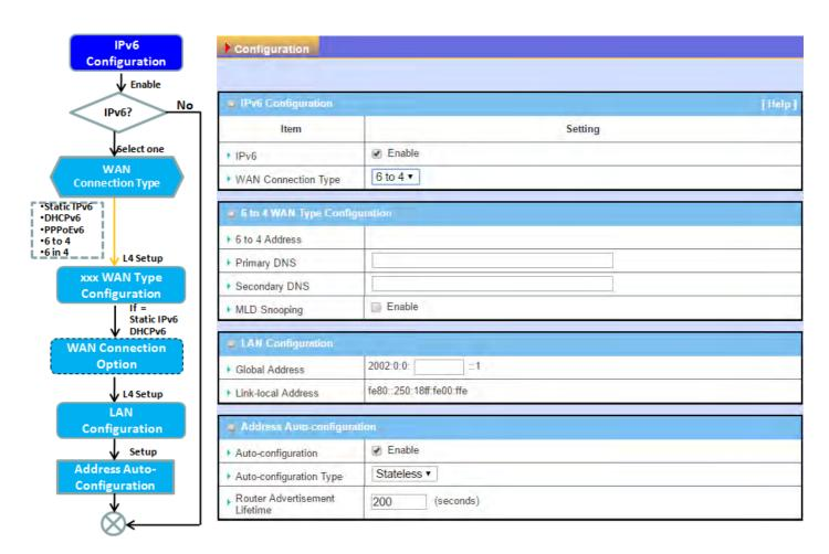
The **IPv6 Configuration** setting allows user to set the IPv6 connection type to access the IPv6 network. This gateway supports various types of IPv6 connection, including **Static IPv6**, **DHCPv6**, and **PPPoEv6**
