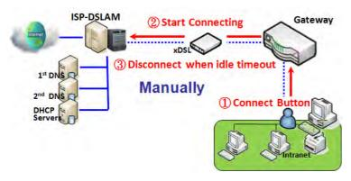
Manually: This gateway won't start to establish WAN connection until you press "Connect" button on web UI. After normal data transferring between LAN and WAN sides, this gateway will disconnect WAN connection if idle time reaches value of Maximum Idle Time.
