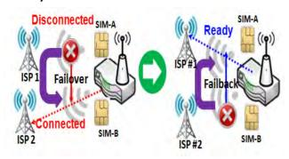
With Failback option enabled, "SIM-A First" scenario is used to connect when the connection is broken, gateway system will switch to use SIM-B. And when SIM-A connection is recovered, it will switch back to use original SIM-A card
