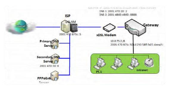
Above diagram depicts DHCP IPv6 IP addressing, the DHCPv6 server on the ISP side assigns IPv6 address, IPv6 default gateway address, and IPv6 DNS to client host's automatically.
