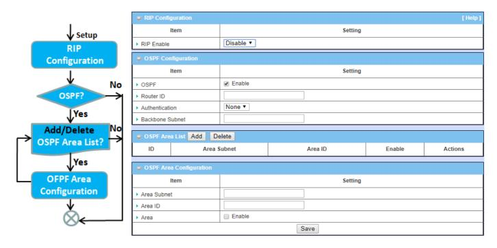
Dynamic Routing, also called adaptive routing, describes the capability of a system, through which routes are characterized by their destination, to alter the path that the route takes through the system in response to a change in network conditions.
