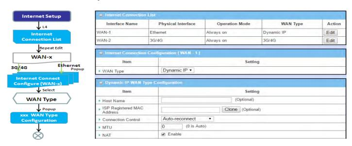
After specifying the physical interface for each WAN connection, administrator must configure their connection profile to meet the dial in process of ISP, so that all client hosts in the Intranet of the gateway can access the Internet.
