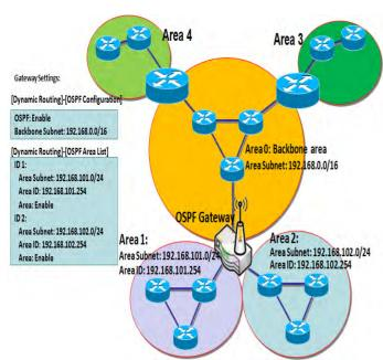
Open Shortest Path First (OSPF) is a routing protocol that uses link state routing algorithm. It is the most widely used interior gateway protocol (IGP) in large enterprise networks. It gathers link state information from available routers and constructs a topology map of the network. The topology is presented as a routing table which routes datagrams based solely on the destination IP address.
