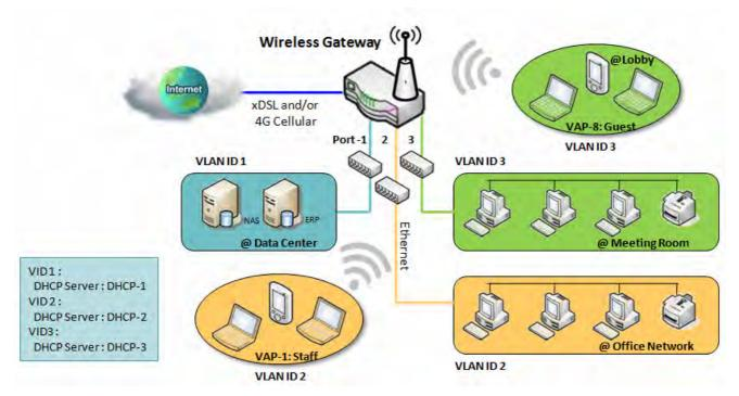
Above is the general case for 3 Ethernet LAN ports in the gateway. But if the device just has one Ethernet LAN port, there will be only one VLAN group for the device. Under such situation, it still supports both the NAT and Bridge mode for the Port-based VLAN configuration.
