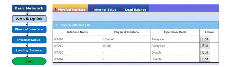
The gateway provides multiple WAN interfaces to let all client hosts in Intranet of the gateway access the Internet via ISP. But ISPs in the world apply various connection protocols to let gateways or user's devices dial in ISPs and then link to the Internet via different kinds of transmit media.
