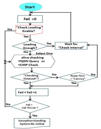
It is necessary to monitor connection status continuous. To do it, "ICMP Check" and "FQDN Query" are used to check. When there is traffic of connection, checking packet will waste bandwidth. Response time of replied packets may also increase. To avoid "Network Monitoring" work abnormally, enabling "Checking Loading" option will stop connection check when there is traffic. It will wait for another "Check Interval" and then check loading again.
