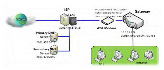
Above diagram depicts the IPv6 IP addressing, type in the information provided by your ISP to setup the IPv6 network.
