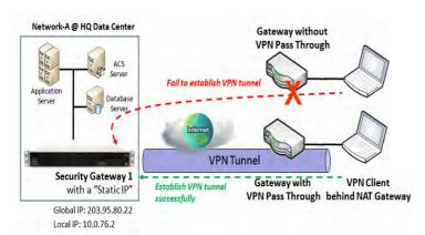
Since VPN traffic is different from that of TCP or UDP connection, it will be blocked by NAT gateway. To support the pass through function for the VPN connections initiating from VPN clients behind NAT gateway, the gateway must implement some kind of VPN pass through function for such application. The gateway support the pass through function for IPSec, PPTP, and L2TP connections, you just have to check the corresponding checkbox to activate it.
