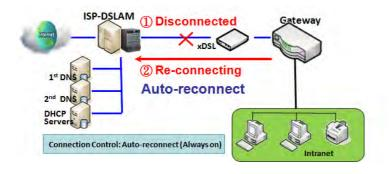
**Auto-reconnect:** This gateway will establish Internet connection automatically once it has been booted up, and try to reconnect once the connection is down. It's recommended to choose this scheme if for mission critical applications to ensure full-time Internet connection.
