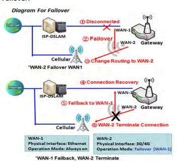
A failover interface is a backup connection to the primary. That means only when its primary WAN connection is broken, the backup connection will be started up to substitute the primary connection.
