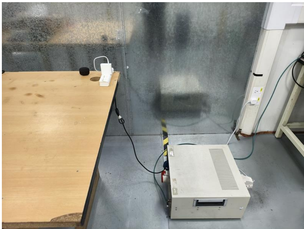
Conducted Emission Test Setup:
