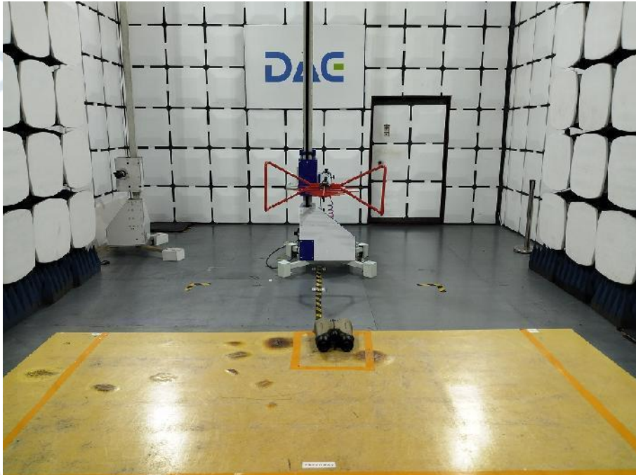
Emissions in frequency bands (below 1GHz)
