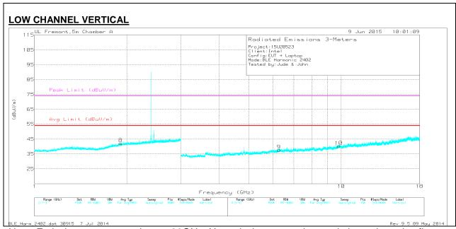
Note: Emission was scanned up to 26GHz; No emissions were detected above the noise floor which was at least 20dB below the specification limit.
