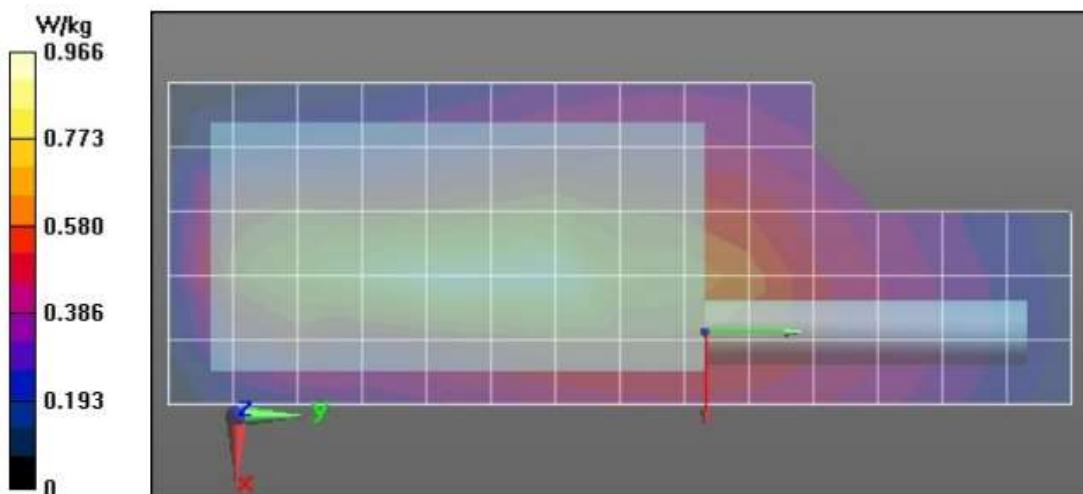
**Shortened scan reflect highest SAR producing configurations and is compared to full scan**
