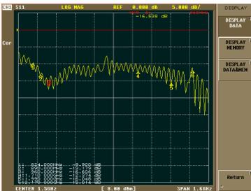
Figure 64:  $|S_{11}|$  sample measurement of a wideband antenna
