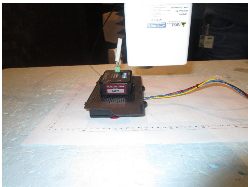
Photograph 6: Measurements in the anechoic chamber, 10cm distance between measurement probe and EUT, Position 2
