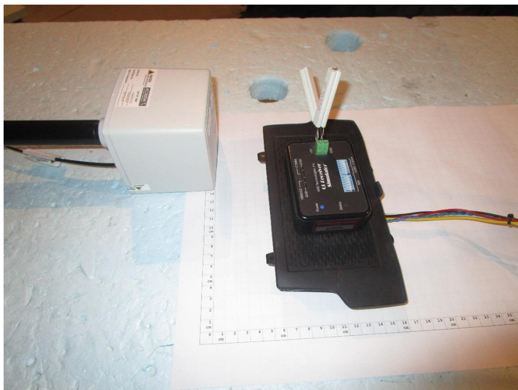
Photograph 13: Measurements in the anechoic chamber, 5cm distance between measurement probe and EUT, Position 5
