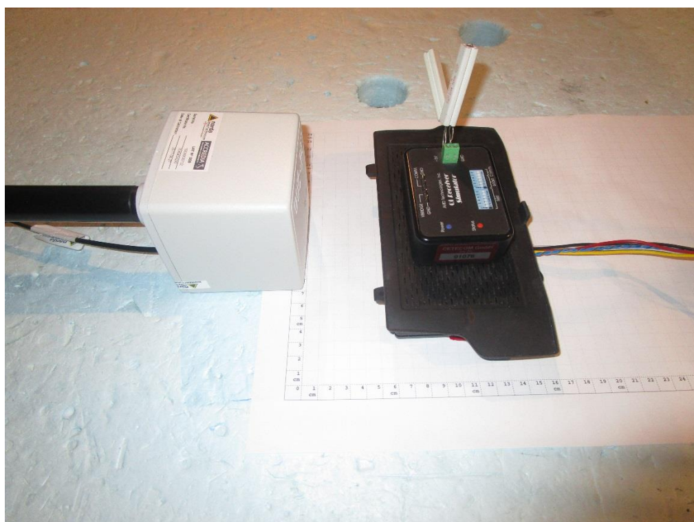
Photograph 7: Measurements in the anechoic chamber, 5cm distance between measurement probe and EUT, Position 3
