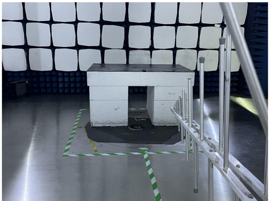
Radiation Emission Test Setup (30MHz to 1GHz)
